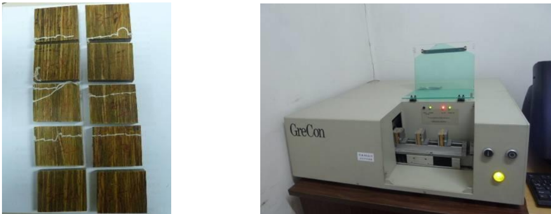
Fig. 2. Specimens of BLVL and profile density analysis apparatus
