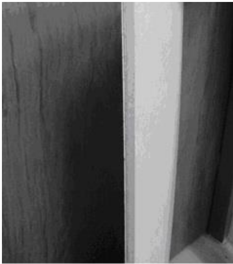
Fig. 3. Photo of the narrow surface of an MDF board veneered on one side
