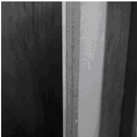
Fig. 5. Photo of the narrow surface of a composite board veneered on one side
