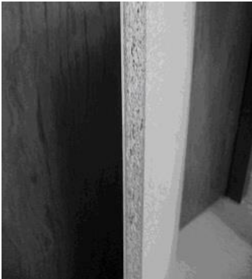
Fig. 1. Photo of the narrow surface of a wood-based panel veneered on one side
