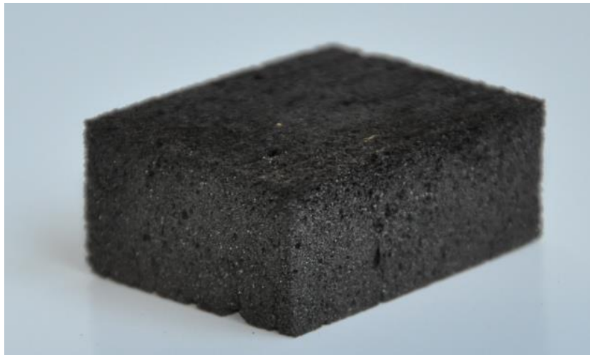
Fig. 2. Formaldehyde-free tannin foam produced with infrared radiation heating system
