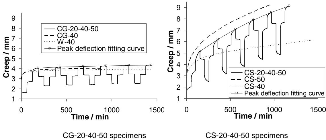
**Fig. 7.** Creep and fitting curves of specimens CG-20-40-50 (left) and CS-20-40-50 (right)
