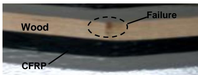
**Fig. 5.** Creep failure of a CS-50 specimen tested in wet condition
