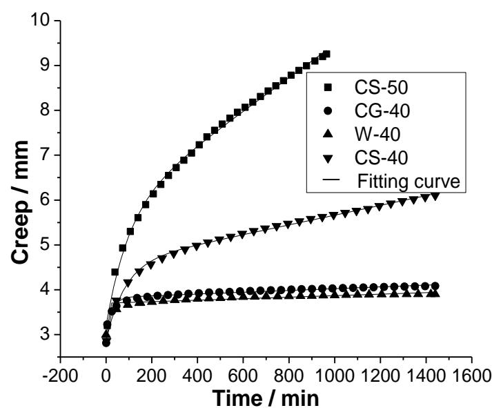
**Fig. 4.** Creep curves and fitting curves of wood and composite specimens at a constant stress level
