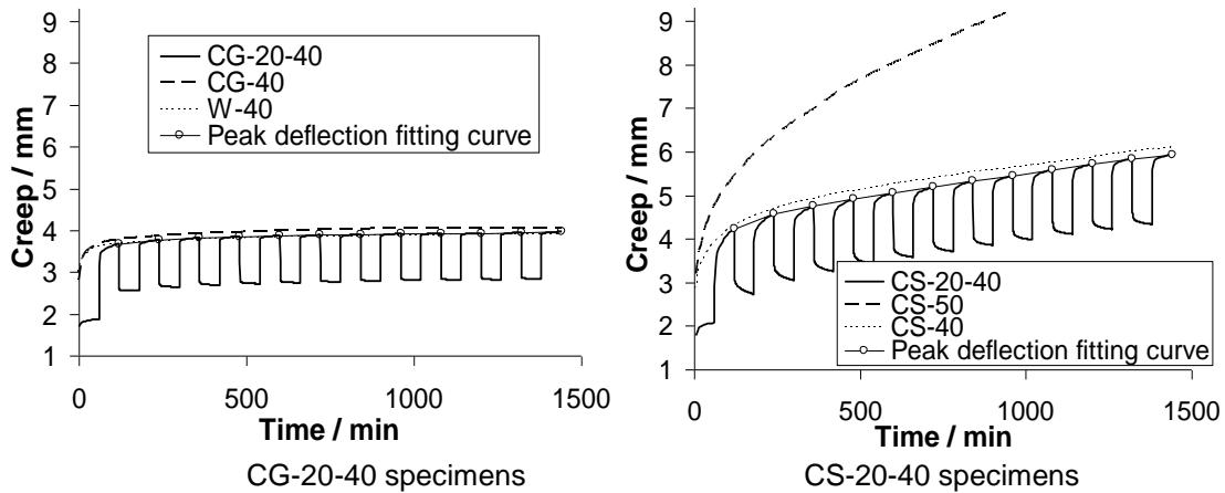
**Fig. 6.** Creep and fitting curves of specimens CG-20-40 (left) and CS-20-40 (right)
