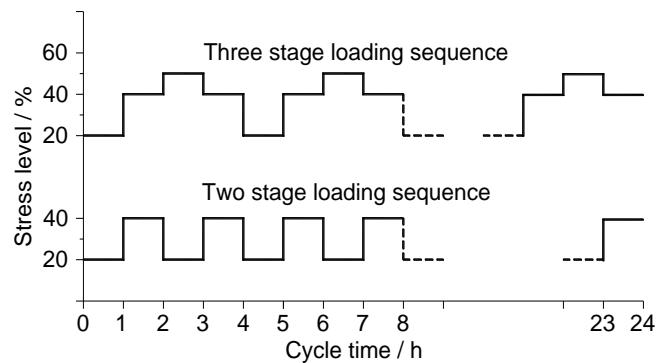
**Fig. 1.** Loading schedules used in creep tests
