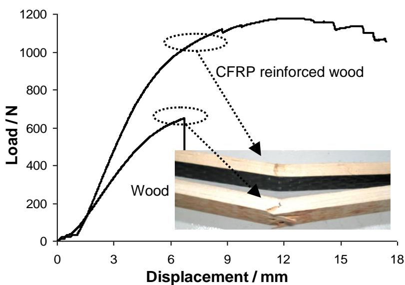
**Fig. 3.** Typical load-deflection curves of wood and composite specimens in bending
