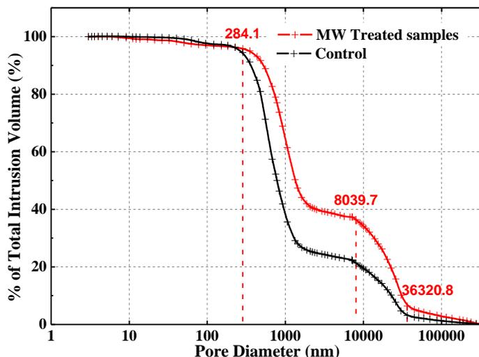
**Fig. 3.** Percentage of intrusion volume *versus* pore diameter of MW-treated and control samples
