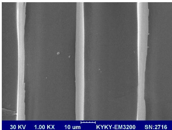
e) Cell wall of tracheids in control samples (x1000)
