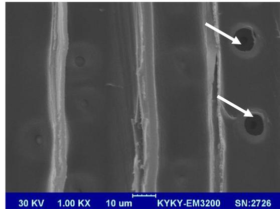
d) Pit membranes in MW-treated samples (x1000)
