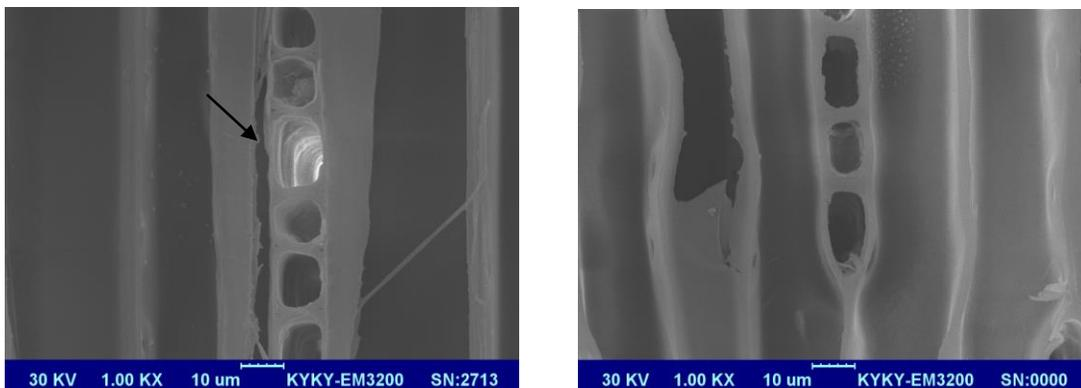
a) Microchecks located at the intercellular layer of ray cells and longitudinal tracheids in MW-treated samples (20 kW, 40% to 60%, 60 s) ( $\times 1000$ )
