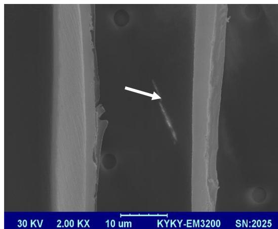
g) Microchecks in cell wall of MW-treated samples (x2000)
