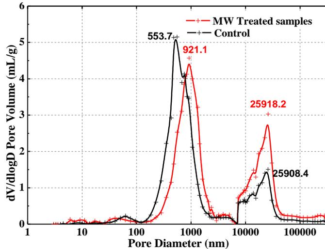
**Fig. 4.** Log differential intrusion *versus* pore diameter of MW-treated and control samples
