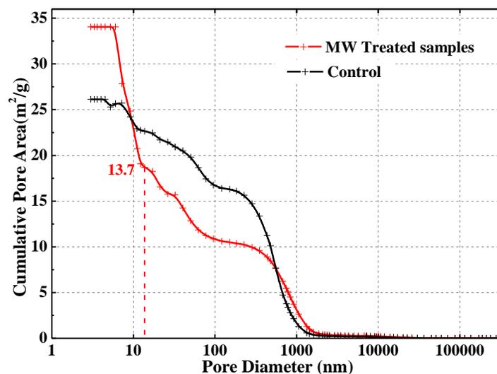
**Fig. 5.** Cumulative pore area *versus* pore diameter of MW-treated and control samples
