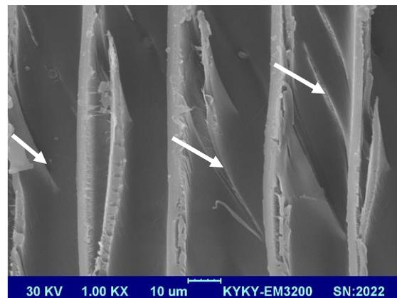
f) Checks in cell wall of tracheids in MW-treated samples (x1000)
