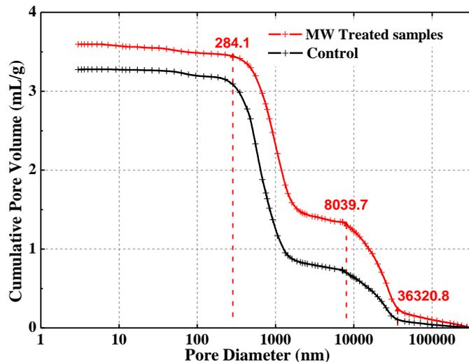
**Fig. 2.** Cumulative pore volume versus pore diameter of MW-treated and control samples
