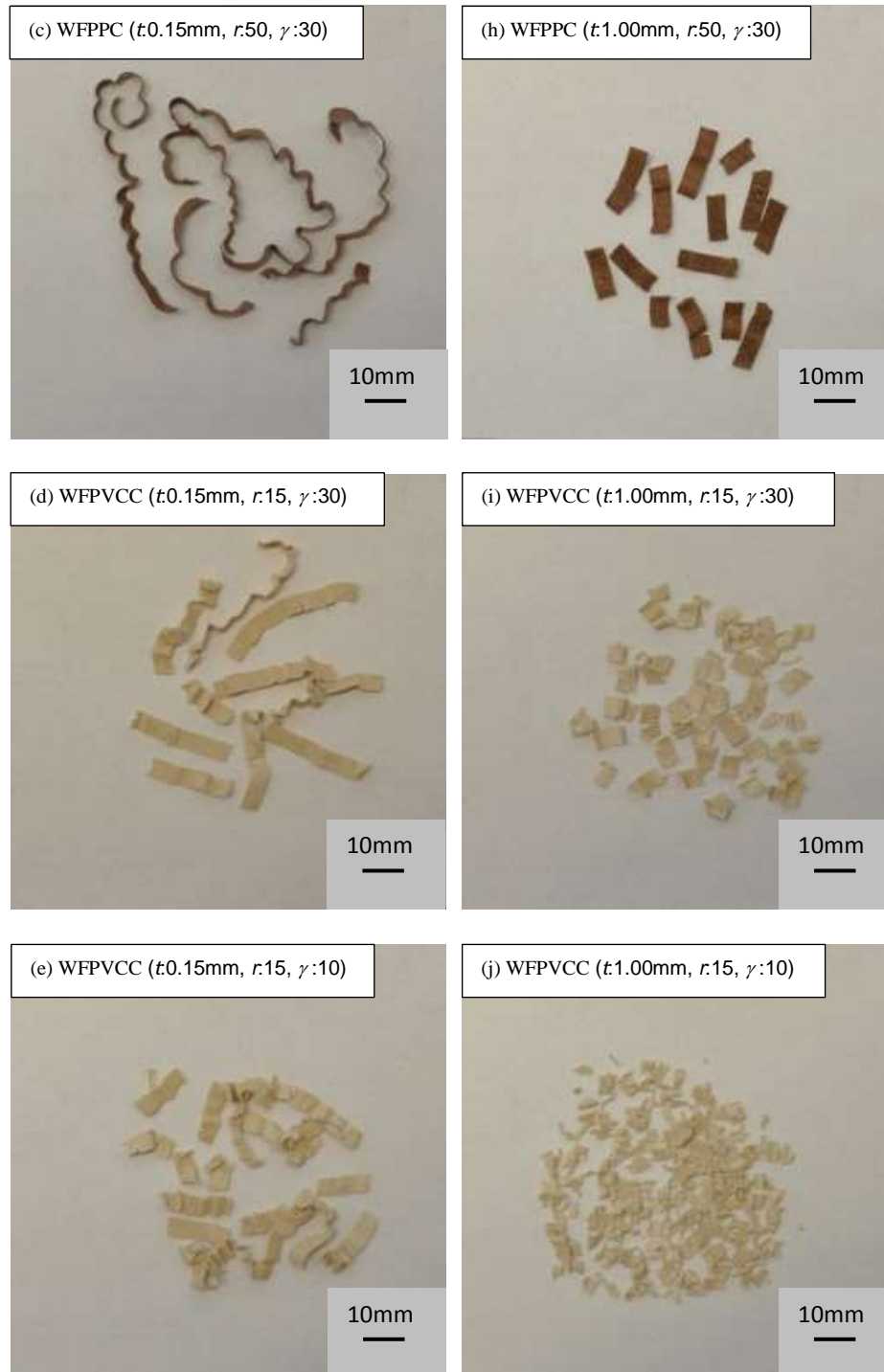
Fig. 8 (c-e & h-j). Chip morphology during cutting of WFPEC (a,f), WFPPC (b, c, g and h) and WFPVCC (d, e, i and j) at t=0.15 and 1 mm, at v=15 m/s
