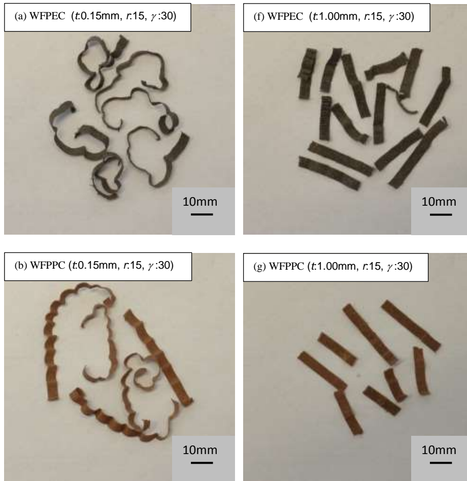
Fig. 8 (a, b, f, g). Chip morphology during cutting of WFPEC (a,f), WFPPC (b, c, g and h) and WFPVCC (d, e, i and j) at t=0.15 and 1 mm, at v=15 m/s
