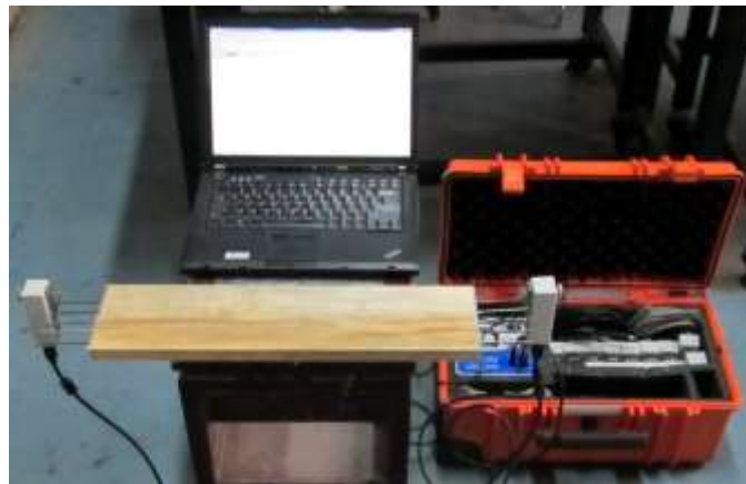
Fig. 2. Experimental set-up for stress wave velocity measurements
