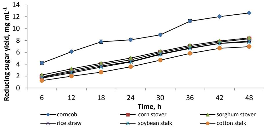
Fig. 1. Reducing sugar yield per mL enzymatic hydrolyzate of pretreated agricultural residues
