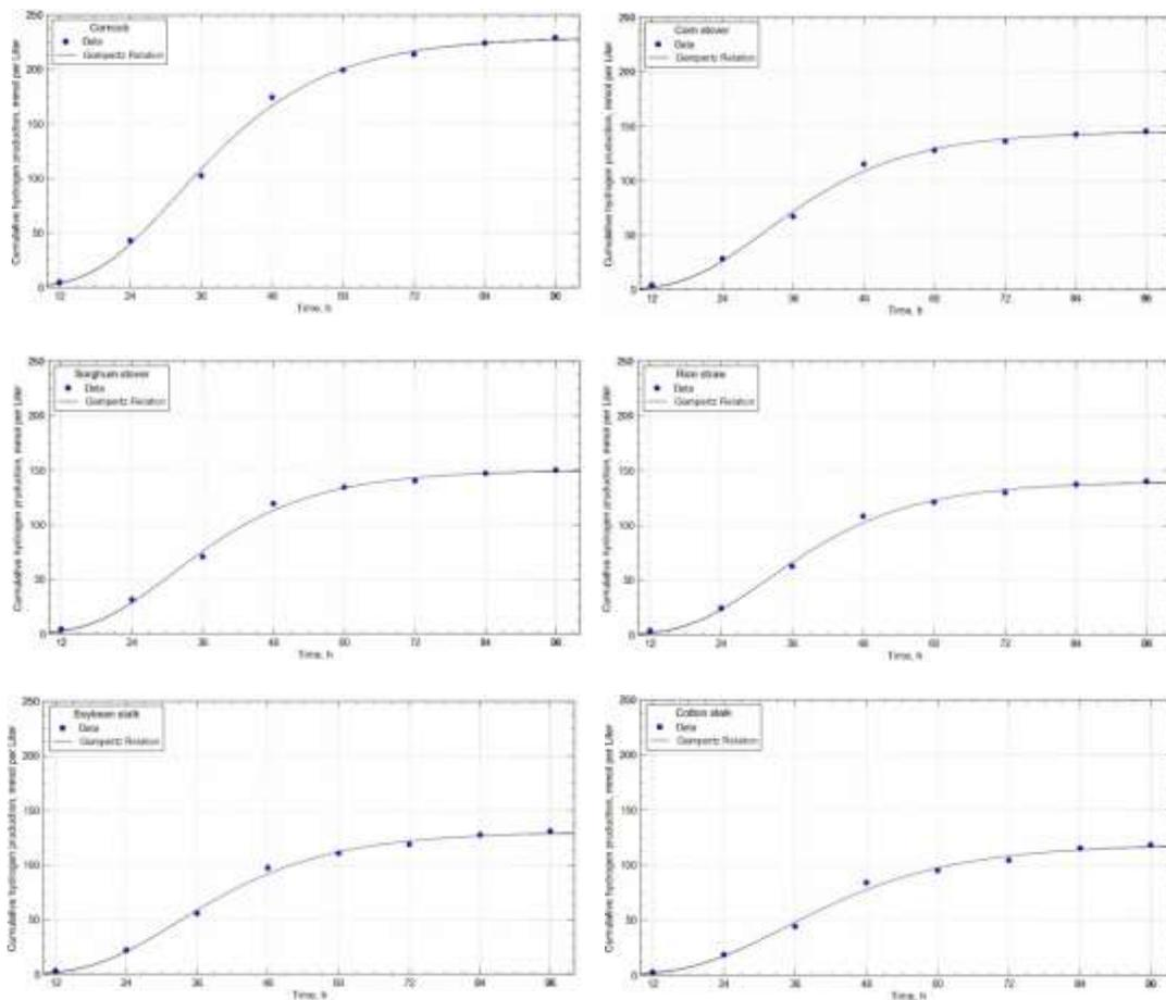
Fig. 2. Cumulative H<sub>2</sub> yield per liter culture versus time of pretreated agricultural residues hydrolyzate
