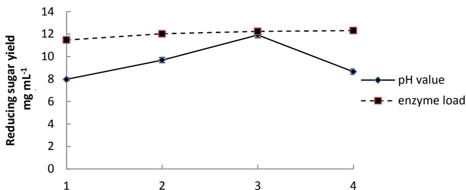
**Fig. 4.** Reducing sugar yield per mL enzymatic hydrolysate of immobilized enzyme at different enzyme loads and pH values (1, 2, 3, 4 represent four levels for each factor, such as pH value of 3.6, 4.2, 4.8, 5.4 and enzyme load of 20, 300, 400, 500 mg, respectively)
