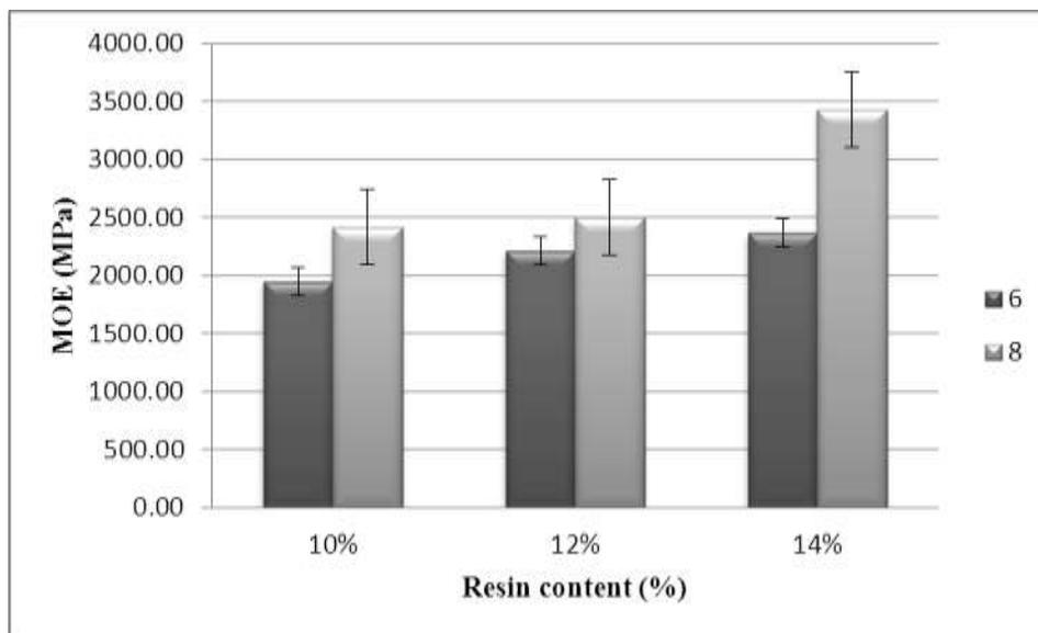
**Fig. 2.** Modulus of elasticity of samples manufactured with different refining conditions (pressure 6 and 8 bar) and resin contents
