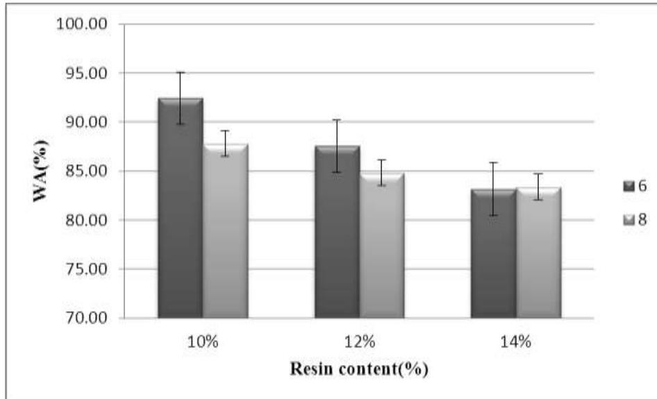
**Fig. 4.** Water absorption of samples manufactured with different refining conditions (pressure 6 and 8 bar) and resin contents
