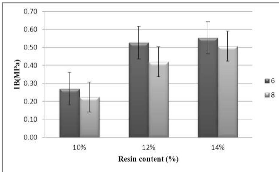
**Fig. 3.** Internal bonding of samples manufactured with different refining conditions (pressure 6 and 8 bar) and resin contents
