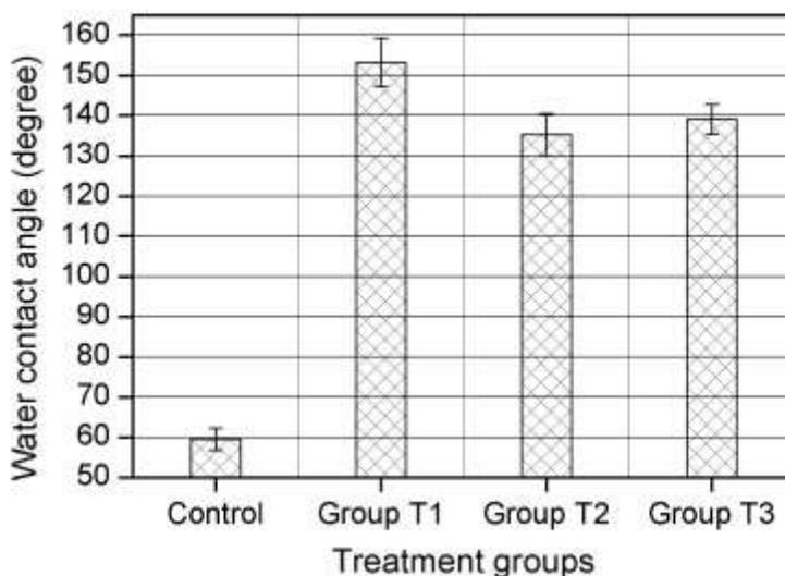
**Fig. 1.** Contact angles of water on treated and untreated wood sample surfaces
