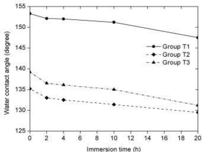
**Fig. 2.** Water contact angles as a function of water immersion time for TiO<sub>2</sub> gel/acacia hybrid wood composites
