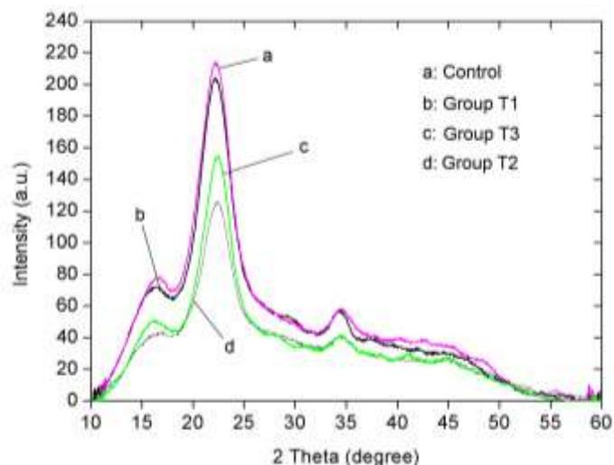
Fig. 4. XRD patterns of different wood samples
