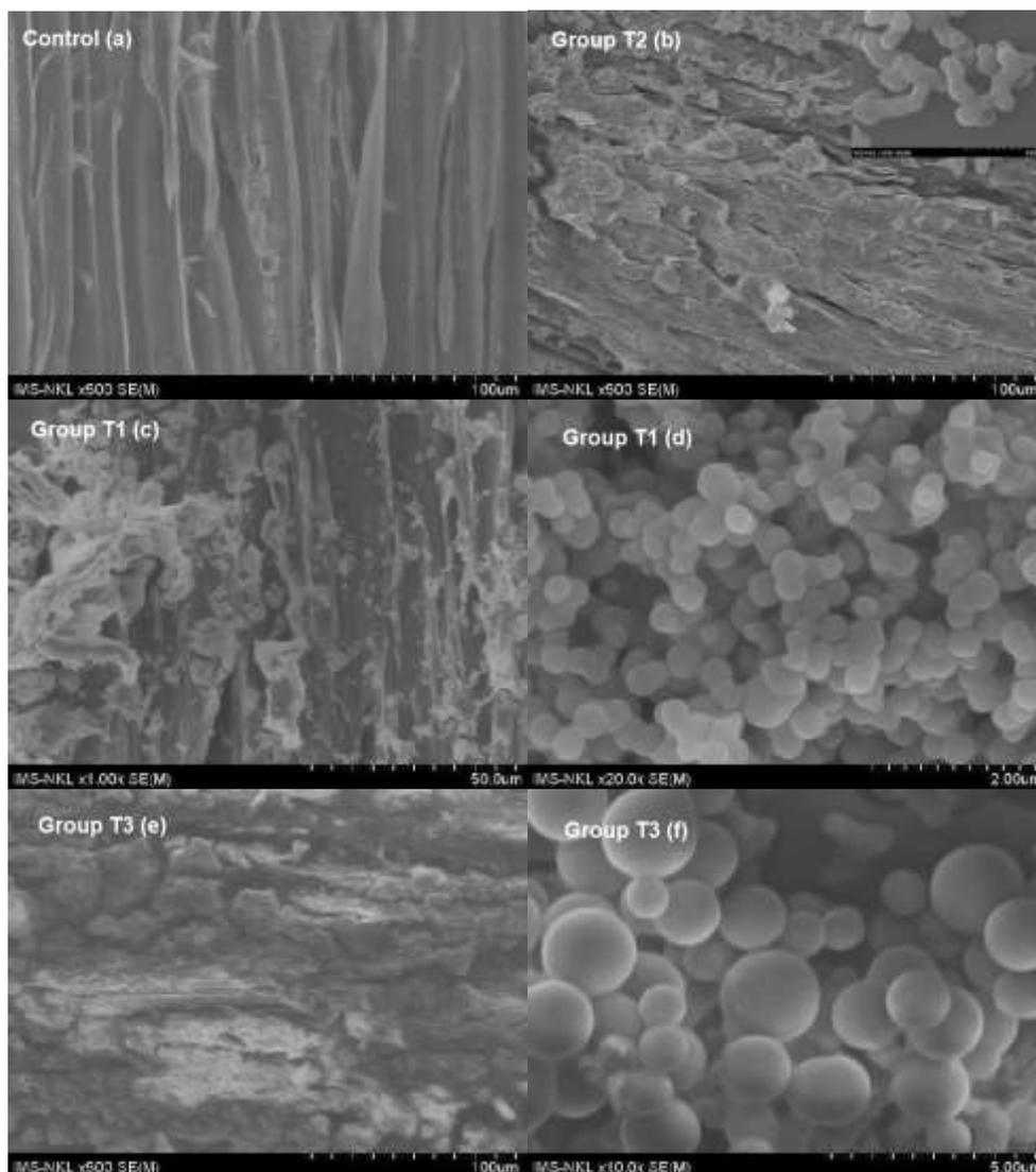
Fig. 3. FE-SEM images of TiO<sub>2</sub>-treated acacia hybrid wood at different magnifications
