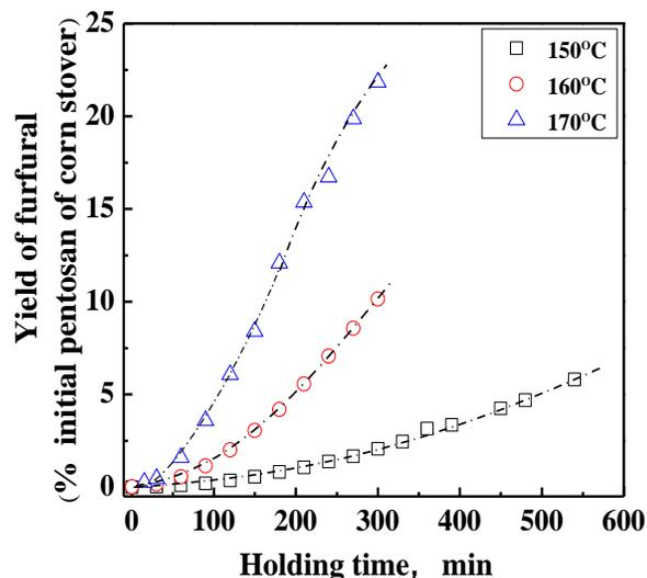
Fig. 6. Effect of temperature and holding time on the yield of furfural
