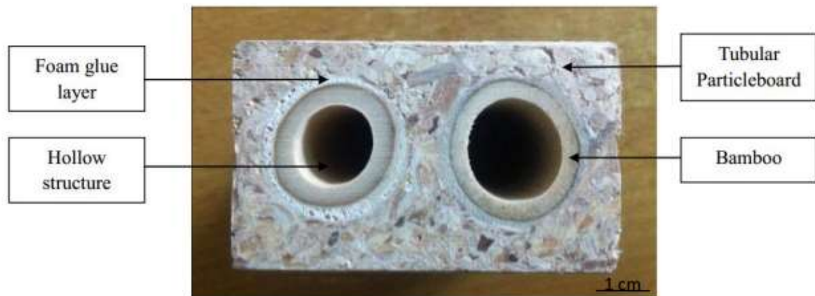
Fig. 2. Cross section of BREP for the compression strength test
