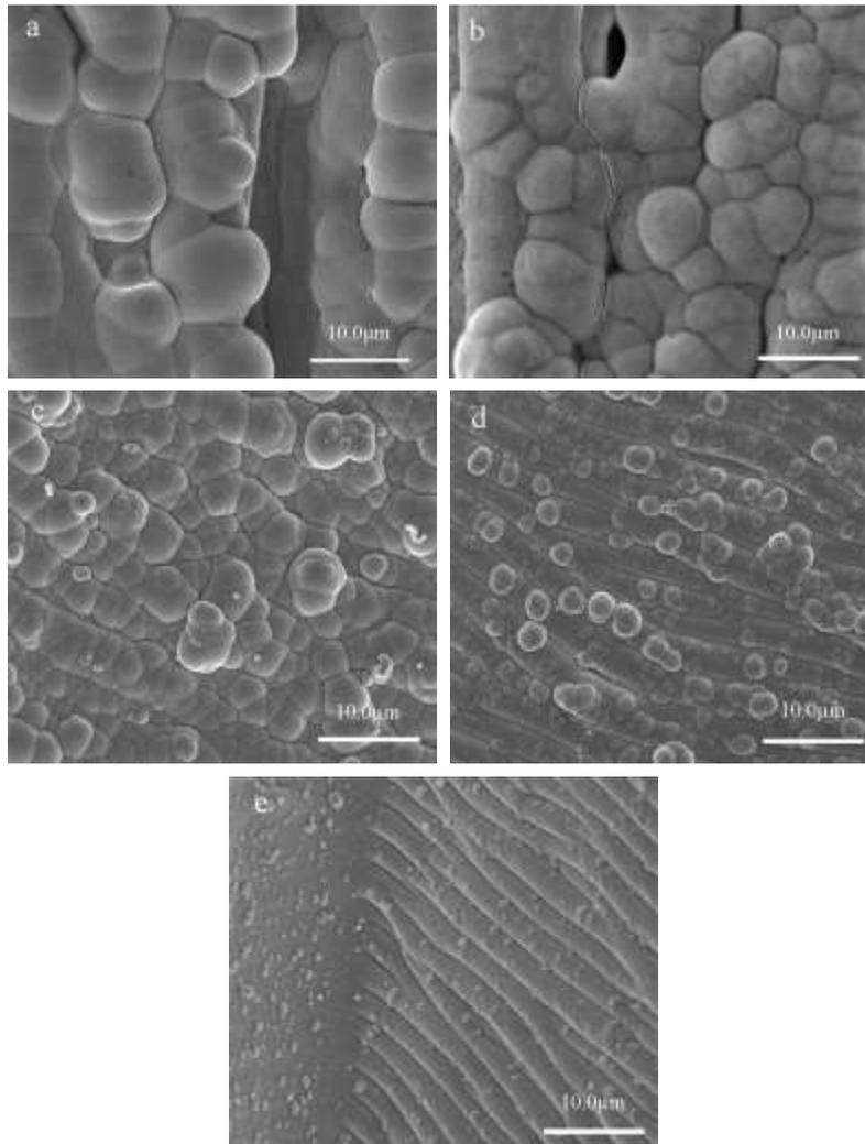
**Fig. 5.** SEM images of Ni-Cu-P-coated veneers with varying copper content: (a) 3.96 wt%, (b) 7.38 wt%, (c) 8.62 wt%, (d) 15.62 wt%, and (e) 20.73 wt%
