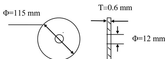
**Fig. 1.** Samples used for testing electromagnetic shielding effectiveness
