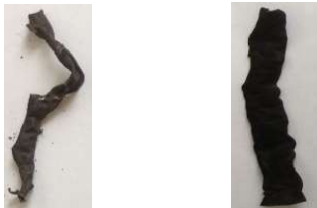
(a) Residue of paper with filler 1 (b) Residue of paper with filler 2
