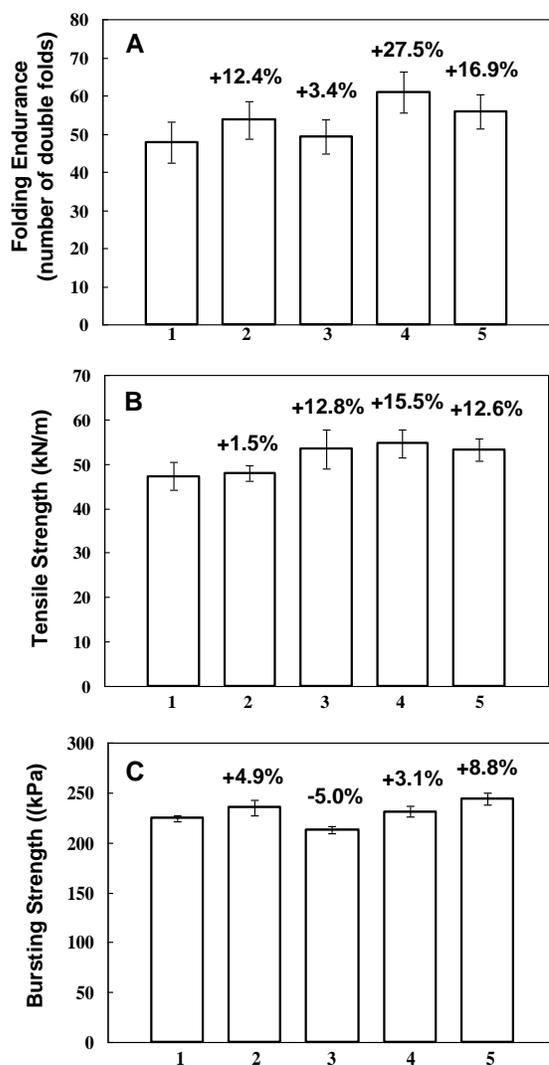
**Fig. 5.** The effect of four engineered double CBMs on the paper's folding endurance (A), tensile strength (B), and bursting strength (C). 1, control paper; 2-5, papers treated with CBM3-GS-CBM1, CBM3-NL-CBM1, CBM3-GS-CBM3, and CBM1-NL-CBM1, respectively.
