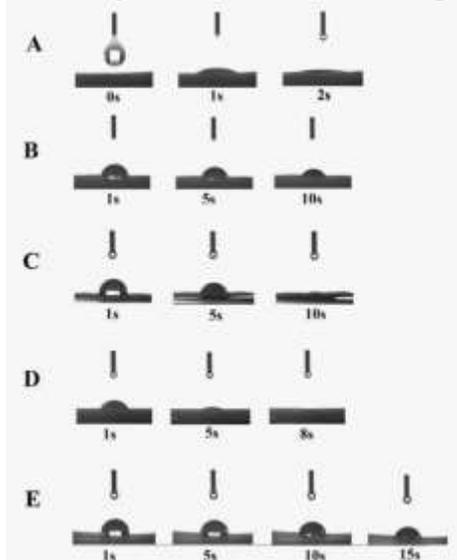
**Fig. 6.** The effect of double CBMs on the wettability of treated papers: A. control paper; B. CBM3-GS-CBM1 treated paper; C. CBM3-NL-CBM1 treated paper; D. CBM3-GS-CBM3 treated paper; E. CBM1-NL-CBM1 treated paper
