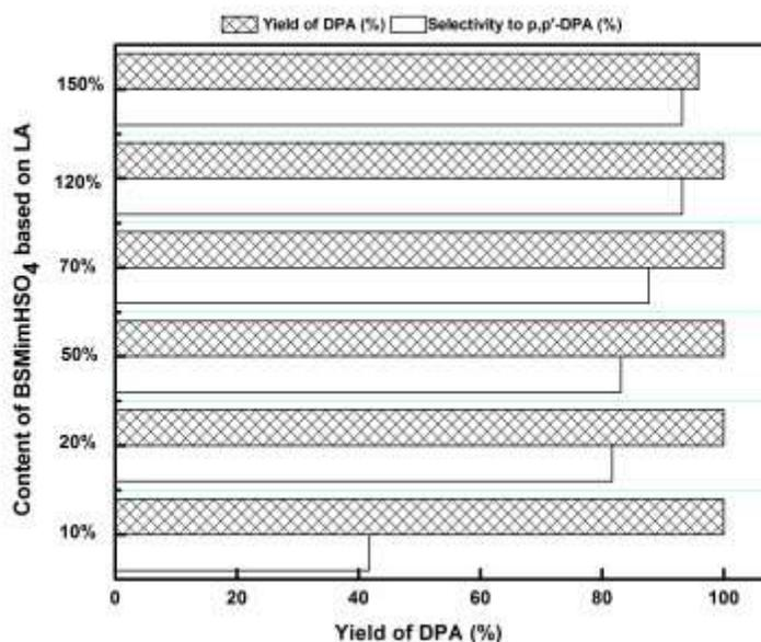
Fig. 4. Effect of the [BSMim]HSO<sub>4</sub> amount on the condensation of phenol with LA
