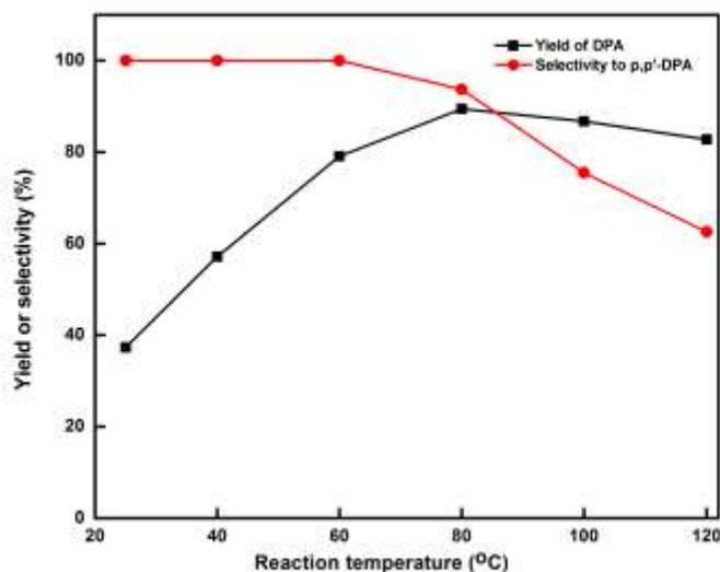
**Fig. 2.** Effect of reaction temperature on the condensation of phenol and LA catalyzed by [BSMim]HSO<sub>4</sub>
