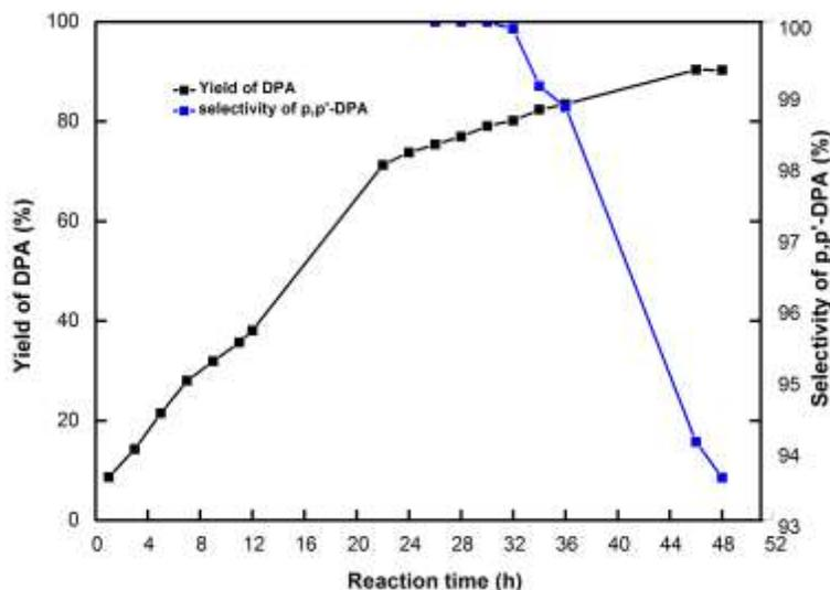
Fig. 1. Effect of reaction time on the condensation of phenol and LA catalyzed by [BSMim]HSO<sub>4</sub>
