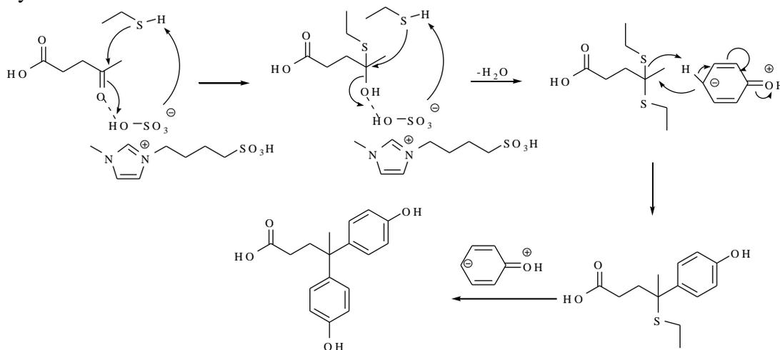
**Scheme 2.** Possible mechanism for thiol involvement in the condensation reaction of phenol and LA catalyzed by [BSMim]HSO<sub>4</sub> ionic liquid
