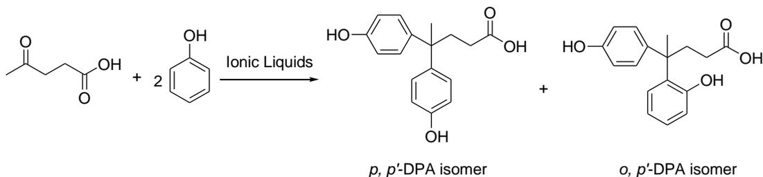
**Scheme 1.** Condensation of LA and phenol to DPA catalyzed by ionic liquid
