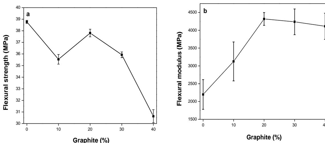
**Fig. 4.** Changes of the flexural strength (a) and flexural modulus (b) of the HDPE/bamboo/graphite composites as a function of graphite content
