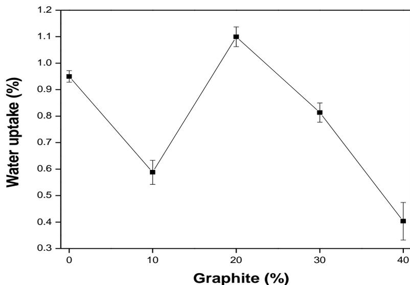
**Fig. 3.** Variation of the water uptake of the HDPE/bamboo/graphite composites as a function of graphite content
