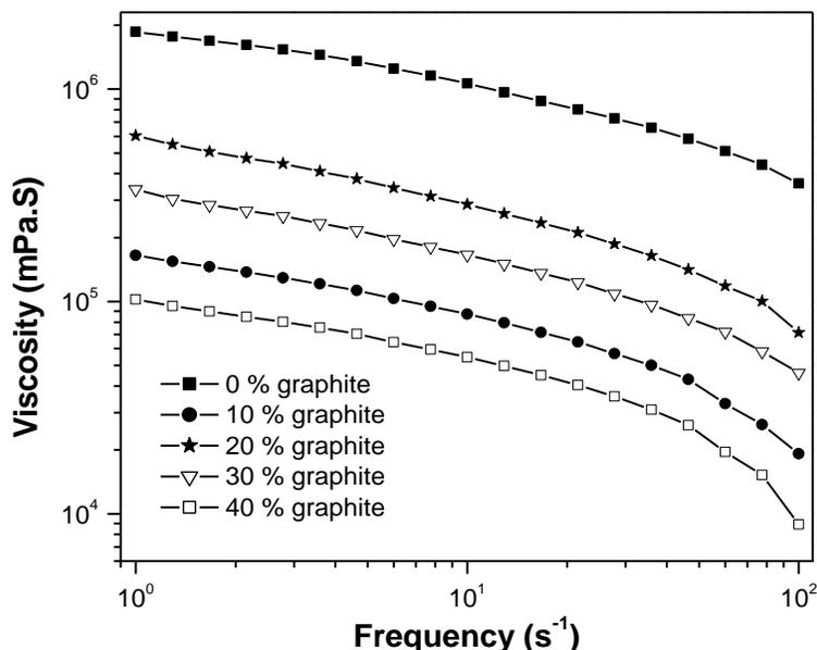
Fig. 2. Viscosity of the HDPE/bamboo/graphite composites with different graphite contents
