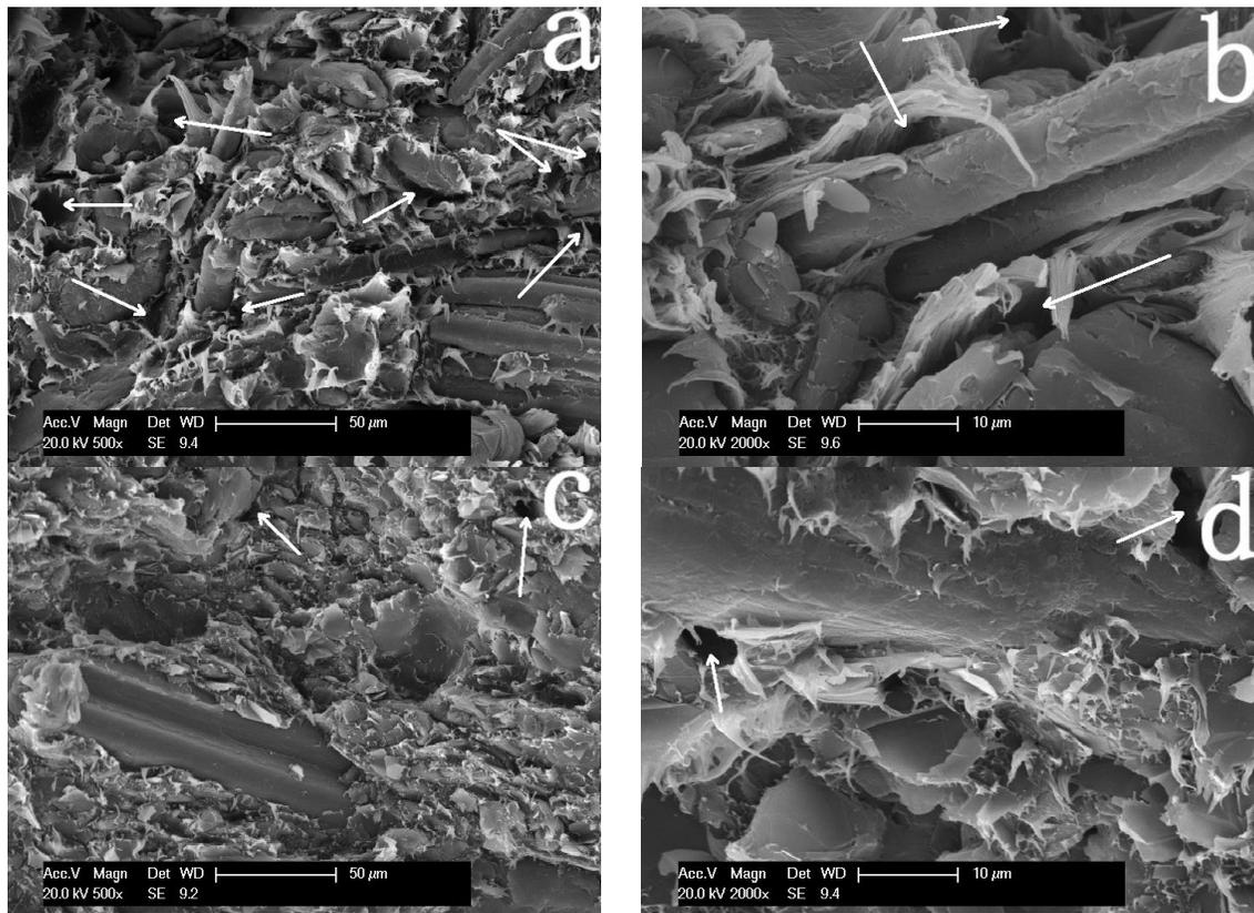
**Fig. 6.** SEM images of the HDPE/bamboo/graphite composite: (a) 20 % of graphite 500x; (b) 20 % of graphite 2000x; (c) 40 % of graphite 500x; (d) 40 % of graphite 2000x.
