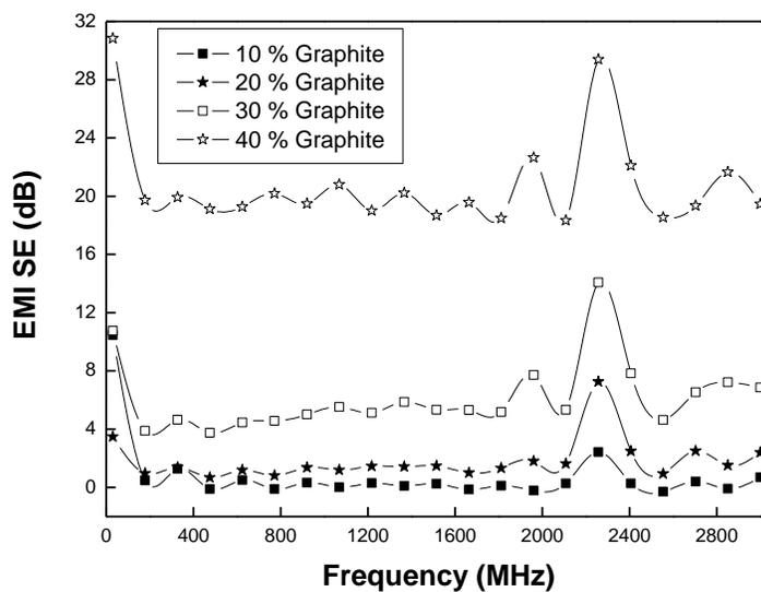
Fig. 7. The EMI SE of HDPE/bamboo/graphite composites as a function of graphite content
