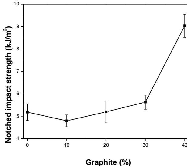
**Fig. 5.** Changes of notched impact strength of the HDPE/bamboo/graphite composites as a function of graphite content
