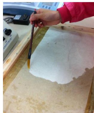
Fig. 4. Surface sizing of dried paper with PVOH
