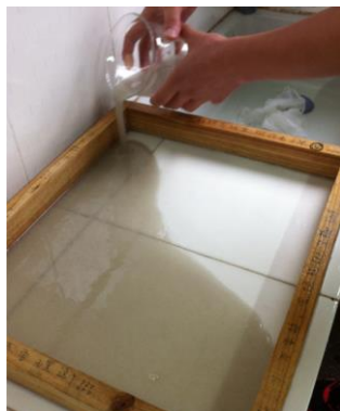
Fig. 3. Liquid suspension poured into sheeting mold
