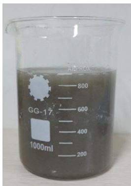
Fig. 2. Uniform liquid suspension of fibers, sludge, and polyacrylamide
