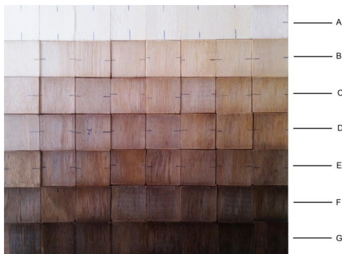
Fig. 4. Color of the modified wood with different dosages of NaOH. (A) untreated wood, (B) treated with 1 wt%, (C) 0.6 wt%, (D) 0.4 wt%, (E) 0.2 wt%, (F) 0.1 wt%, and (G) 0 wt% NaOH. Glyoxal concentration is 20%, (\text{NH}_4)_2\text{S}_2\text{O}_8 dosage is 2 wt% (final solution), glycol to glyoxal ratio is 1:2, and curing temperature is 120 °C
