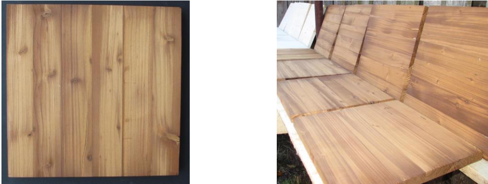
Fig. 1. Solid wood panels obtained from small-diameter spruce wood semi-products, heat-treated within the present research
