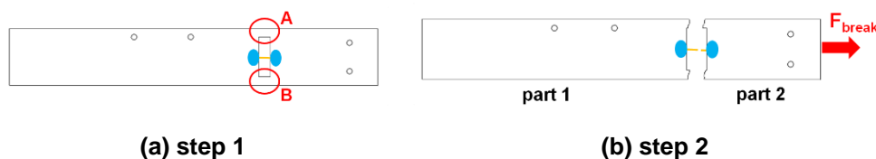
Fig. 4. Determination of the single fiber tensile strength
