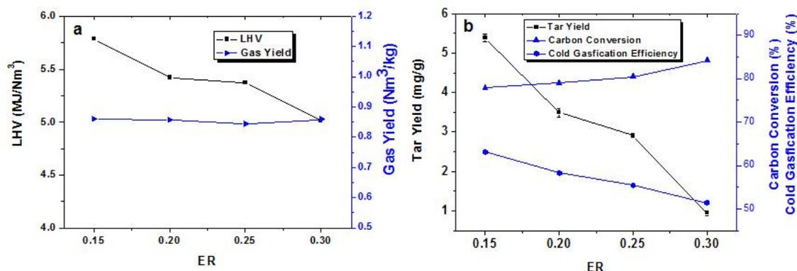
Fig. 7. Effects of ER on gas indices: (a) LHV and gas yield, (b) carbon conversion, cold gas efficiency, and tar yield
