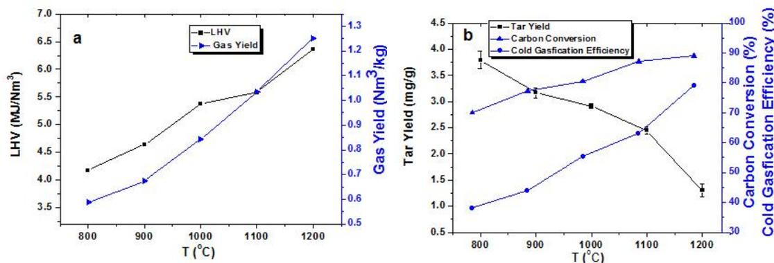
**Fig. 5.** Effects of temperature on gas indices: (a) LHV and gas yield, (b) carbon conversion, cold gas efficiency, and tar yield
