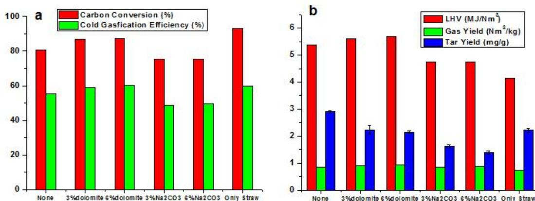
**Fig. 9.** Effects of catalysts on gas indices: (a) carbon conversion and cold gas efficiency, (b) LHV, gas yield, and tar yield
