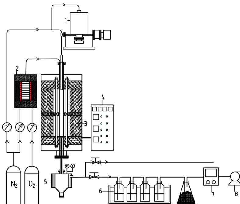
**Fig. 1.** Sketch of the experimental system; (1) feeder, (2) preheater, (3) entrained-flow reactor, (4) temperature controller, (5) hopper, (6) tar collection system, (7) gas flow meter, and (8) pump
