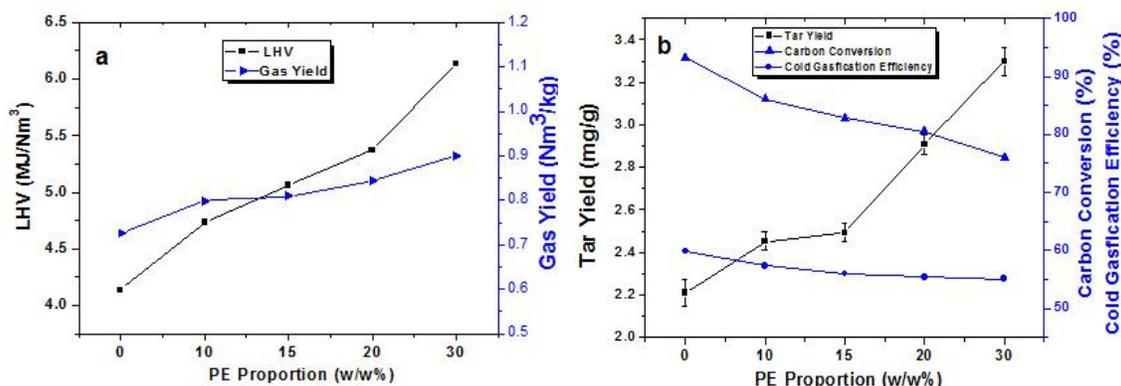
**Fig. 3.** Effects of PE proportion on gasification indices: (a) LHV and gas yield, (b) carbon conversion, cold gas efficiency, and tar yield
