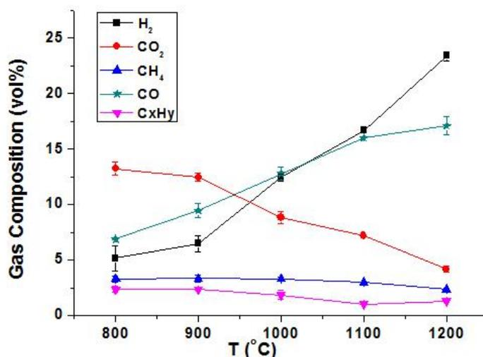
Fig. 4. Effects of temperature on gas composition
