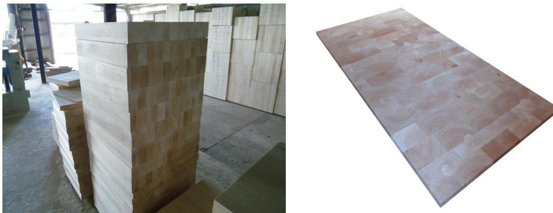
**Fig. 1.** Large glued block of basla (left) and end-grain panel (right) commonly exported from PNG as a core catalyst material
