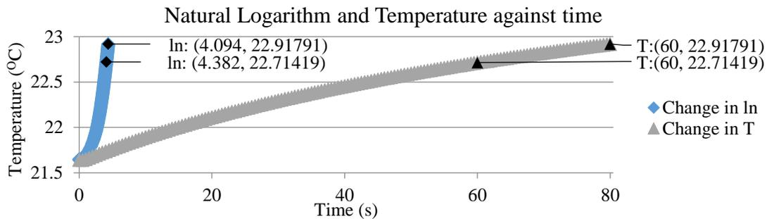
**Fig. 3.** Change in natural logarithm and temperature against time**Table 2.** Data Used to Calculate the TC for Test 1, Sample L Long, Trial 1
