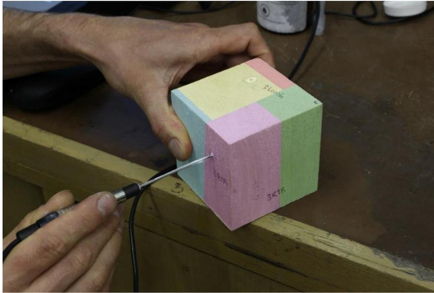
**Fig. 5.** End-grain sample consisting of five different densities (colour used to identify different laminated components of balsa used to manufacture the end-grain sample)
