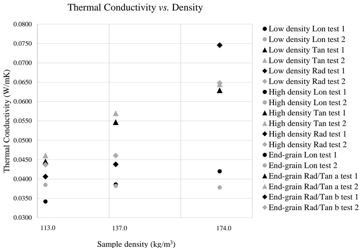
**Fig. 4.** Mean calculated TC from tests 1 and 2 graphed against density to show the effect density has on TC
