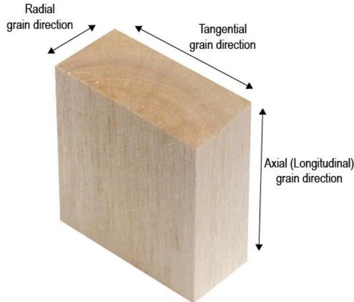
**Fig. 2.** Labeled balsa sample identifying wood grain direction
