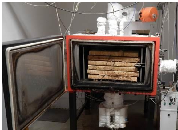
Fig. 2. Laboratory thermal furnace S250/03 filled with spruce boards
