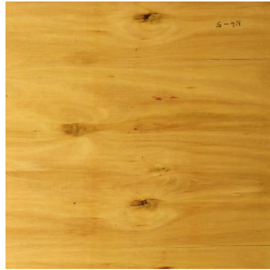
Fig. 3. Example of the visual quality of C-grade veneer
