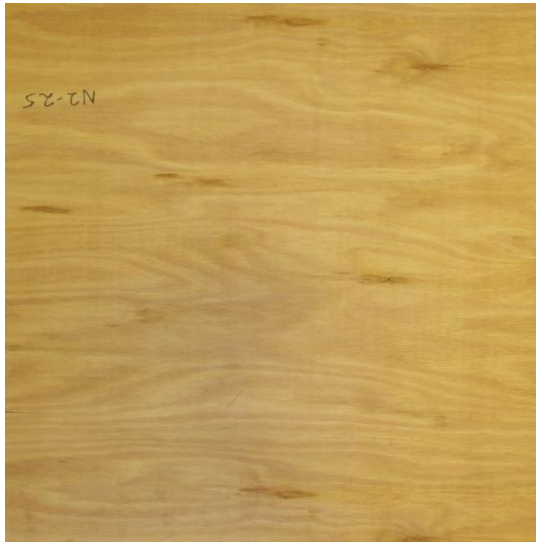
Fig. 2. Example of the visual quality of B-grade veneer
