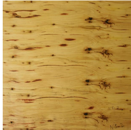
Fig. 5. Example of the visual quality of F-grade (or reject) veneer
