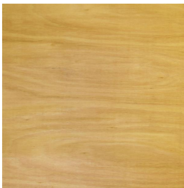
Fig. 1. Example of the visual quality of A-grade veneer
