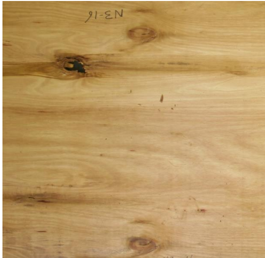
Fig. 4. Example of the visual quality of D-grade veneer
