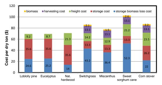
**Fig. 1.** Biomass delivered cost for each feedstock, considering 5% covered area and annual supply of 453,597 dry ton *per* year (Gonzalez *et al.* 2011d)
