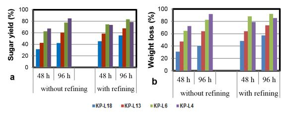
Fig. 6. (a) Sugar yield and (b) weight loss of kraft pretreated and kraft followed by oxygen delignified pine in enzymatic hydrolysis at 48 h and 96 h
