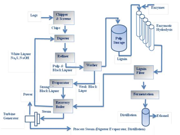
Fig. 8. Conceptual diagram of repurposing a kraft mill for ethanol production
