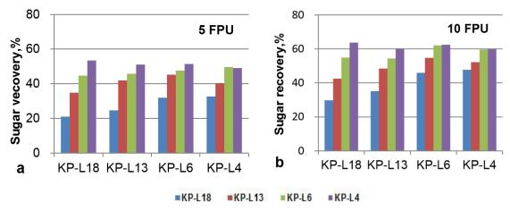
**Fig. 7.** Comparing the sugar recovery of kraft pretreated and kraft pretreated followed by oxygen delignified pine in enzymatic hydrolysis at enzyme loadings of (a) 5 and (b) 10 FPU/g of substrate
