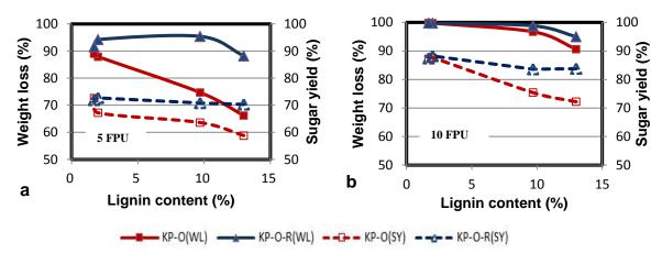
**Fig. 4.** Weight loss and sugar yield of kraft pretreated followed by oxygen delignified pine in enzymatic hydrolysis at enzyme loadings of (a) 5 and (b) 10 FPU/g of substrate (KP-O: kraft pulp with oxygen delignification; KP-O-R: kraft pulp with oxygen delignification and refining.)
