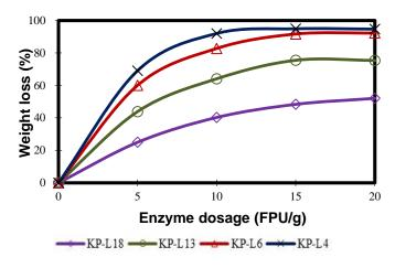
Fig. 2. Effect of enzyme dosage on EH of kraft pulp
