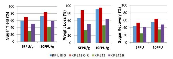
**Fig. 5.** Comparison of EH efficiency at the same lignin content (Any of the pulps having –R attached to the end mean the pulp was refined in PFI prior to enzymatic hydrolysis)
