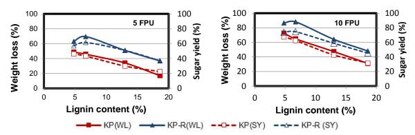
**Fig. 3.** Weight loss and sugar yield of kraft pretreated pine in enzymatic hydrolysis at enzyme loadings of 5 and 10 FPU/g of substrate (KP: kraft pulp, KP-R: kraft pulp with refining, WL: weight loss, SY: sugar recovery)
