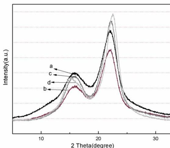
**Fig. 4.** X-ray diffraction patterns of (a) the original particles, (b) holo-cellulose, (c)  $\alpha$ -cellulose, and (d) CNFs
