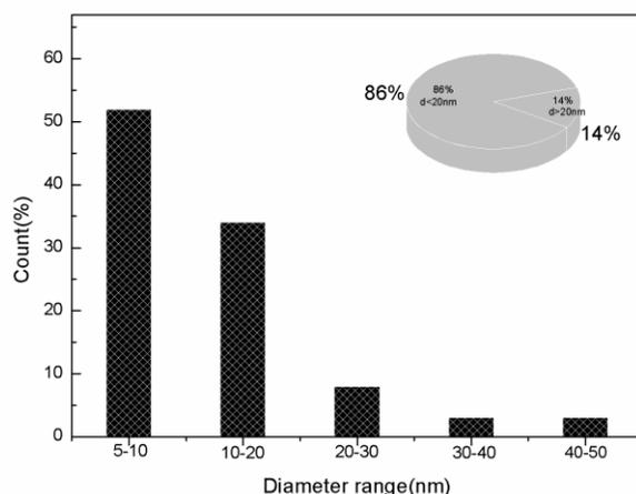
**Fig. 2.** Diameter distribution of the CNFs after a combination of acid treatment and ultrasonication
