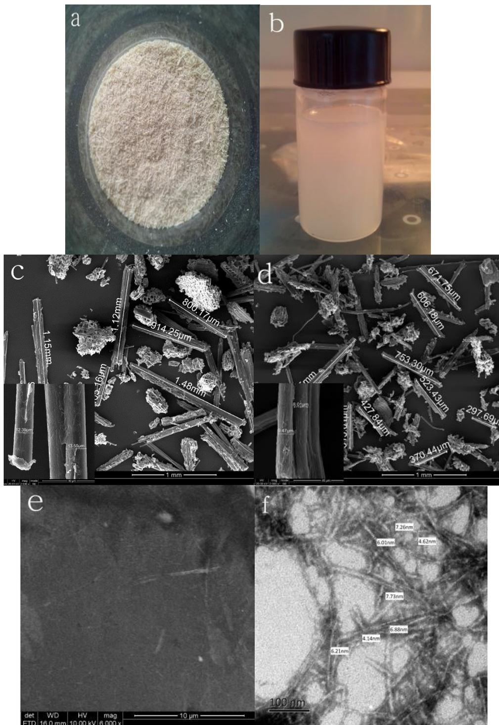
**Fig. 1.** Optical images of (a) the original *Ph. nidularia* Munro particles and (b) CNFs dispersed in water; (c) SEM micrographs of holo-cellulose, (d)  $\alpha$ -cellulose, and (e) CNFs; (f) TEM micrograph of CNFs
