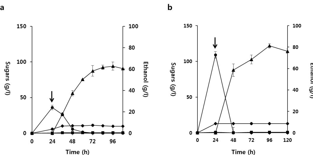
**Fig. 3.** Partial SSF kinetics with pretreated GU containing 12% glucan (a) and 16% glucan (b); ethanol ( $\blacktriangle$ ), glucose ( $\bullet$ ), xylose ( $\blacklozenge$ ), and arabinose ( $\blacksquare$ ). Fermentation was conducted in a 5-L reactor. Arrows indicate cell addition at 24 h. Bars represent standard deviation from three independent experiments
