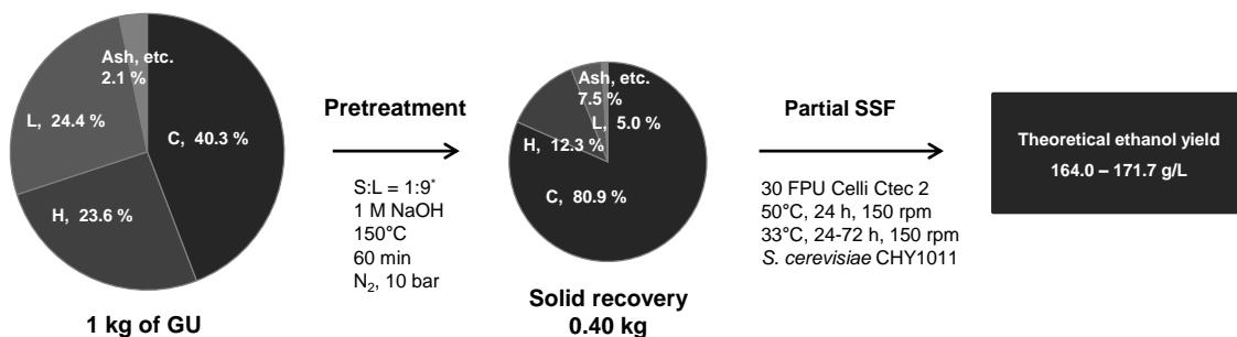
**Fig. 4.** Overall processes based on dry matter content. C = cellulose; H = hemicellulose; and L = lignin. \*S:L = solid:liquid ratio
