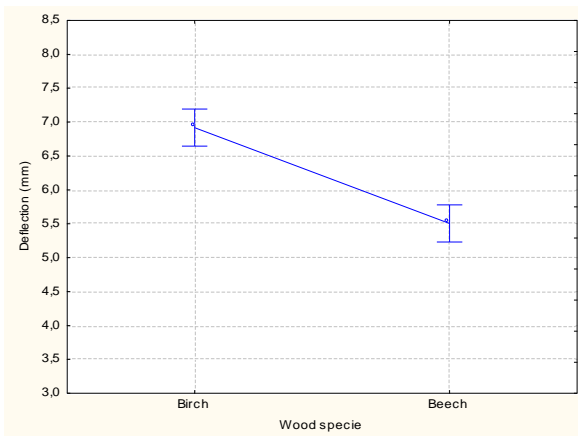
Fig. 5. Effect of wood species type on deflections
