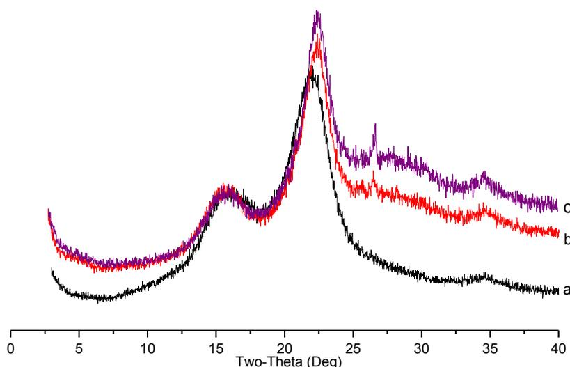
**Fig. 3.** X-ray diffraction spectra of untreated and pretreated bamboo: (a) untreated, (b) pretreated with 1.00% acid at 130 °C for 30 min, and (c) pretreated with 1.00% acid at 150 °C for 30 min
