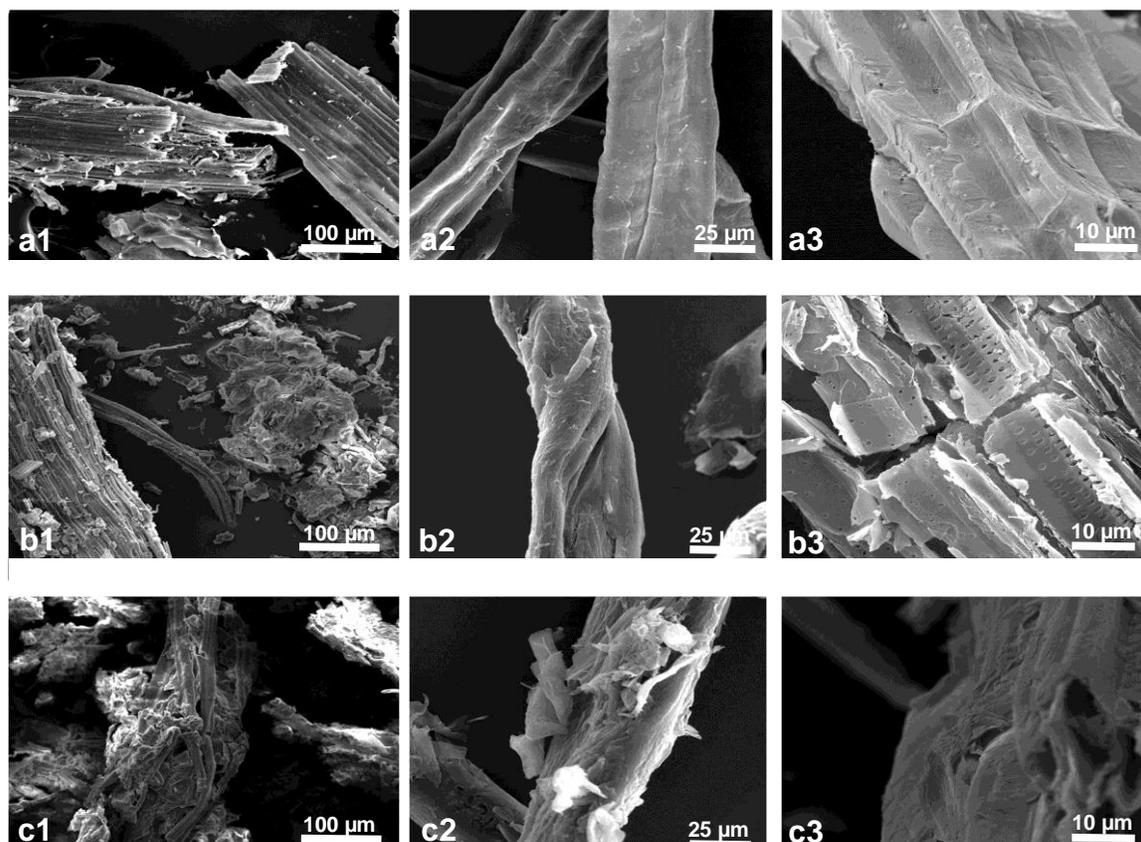
**Fig. 2.** Scanning electron micrographs of untreated and pretreated bamboo: (a) untreated, (b) pretreated with 1.00% acid at 130 °C for 30 min, and (c) pretreated with 1.00% acid at 150 °C for 30 min
