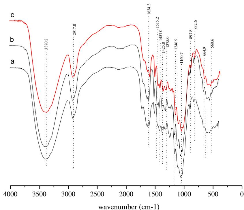
**Fig. 4.** FTIR of untreated and pretreated bamboo: (a) untreated, (b) pretreated with 1.00% acid at 130 °C for 30 min, and (c) pretreated with 1.00% acid at 150 °C for 30 min
