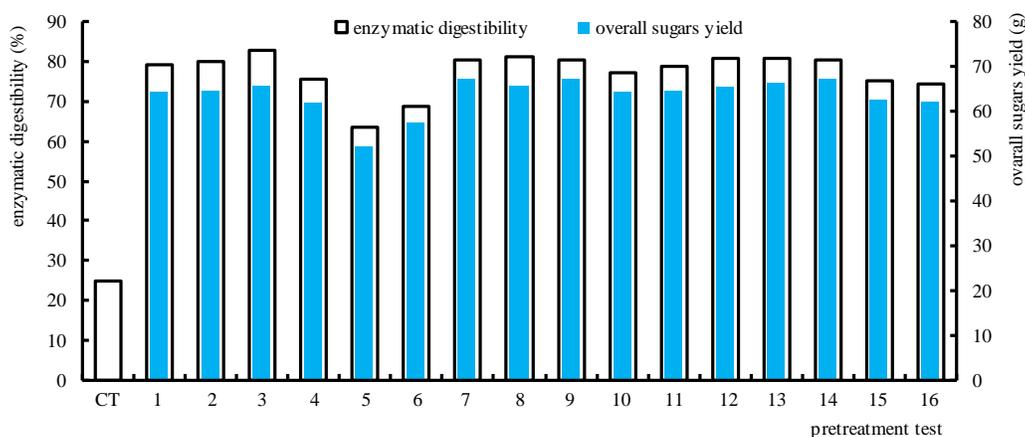
**Fig. 1.** Enzymatic digestibility of untreated sample and pretreated residue under various conditions (see pretreatment test CT, 1-16.)
