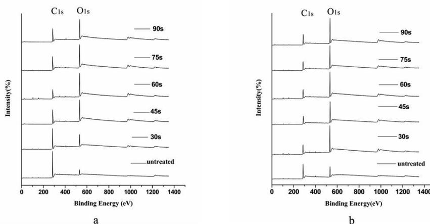
**Fig. 6.** XPS survey spectra of the wheat straw before and after plasma treatment (a- exterior surface; b- interior surface)
