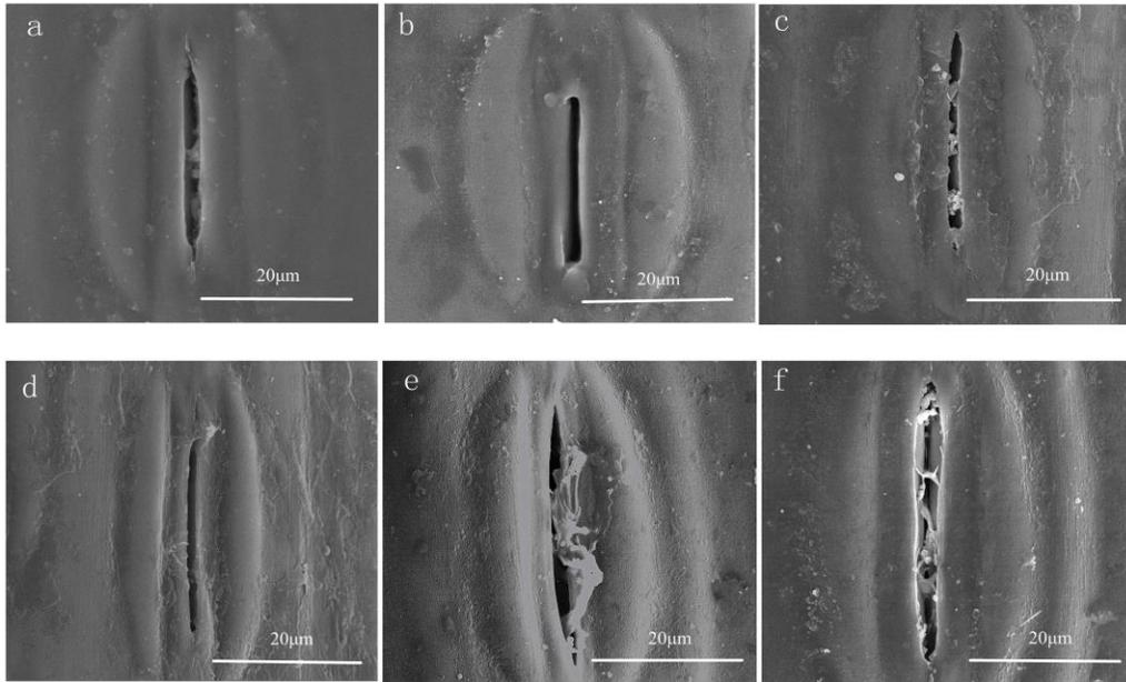
**Fig. 3.** Exterior surfaces of the wheat straw observed under SEM (a- untreated; b- plasma treatment of 30 s; c- plasma treatment of 45 s; d- plasma treatment of 60 s; e- plasma treatment of 75 s; f- plasma treatment of 90 s)
