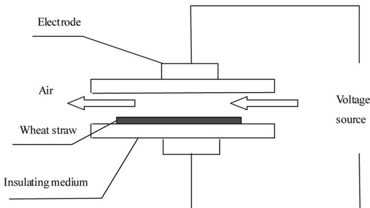
**Fig. 1.** Atmospheric pressure plasma processor
