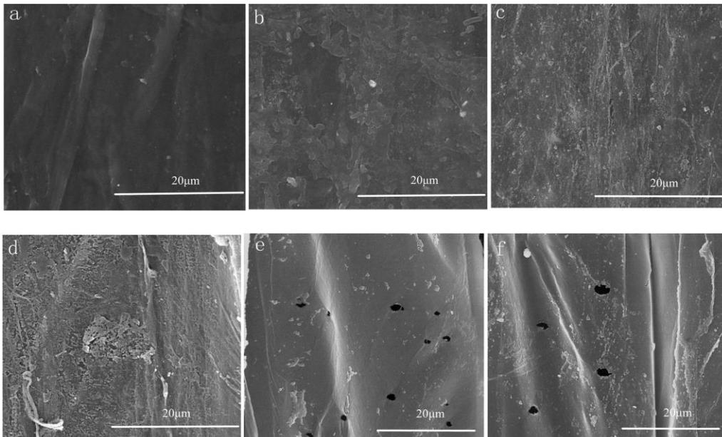
**Fig. 4.** Interior surfaces of the wheat straw observed using SEM (a- untreated; b- plasma treatment of 30 s; c- plasma treatment of 45 s; d- plasma treatment of 60 s; e- plasma treatment of 75 s; f- plasma treatment of 90 s)
