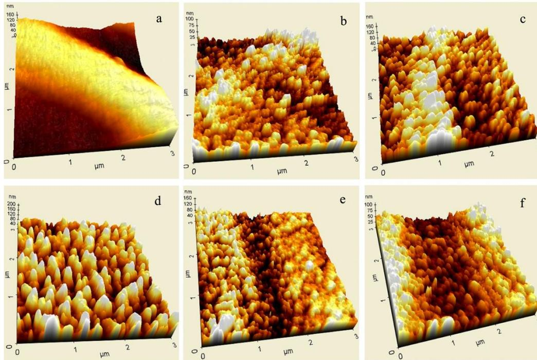
**Fig. 5.** 3D AFM image of wheat straw fibers (a- untreated; b-plasma treatment 30 s; c- plasma treatment 45 s; d- plasma treatment 60 s; e- plasma treatment 75 s; f- plasma treatment 90 s)
