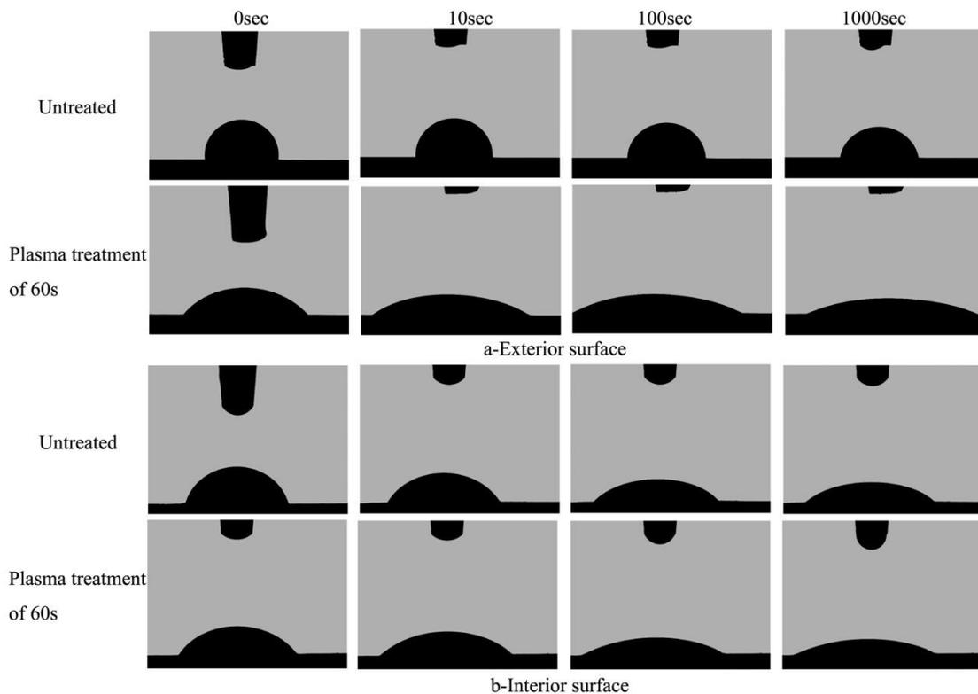
**Fig. 2.** Contact angle changes on the untreated and treated wheat straw surfaces after different wetting periods
