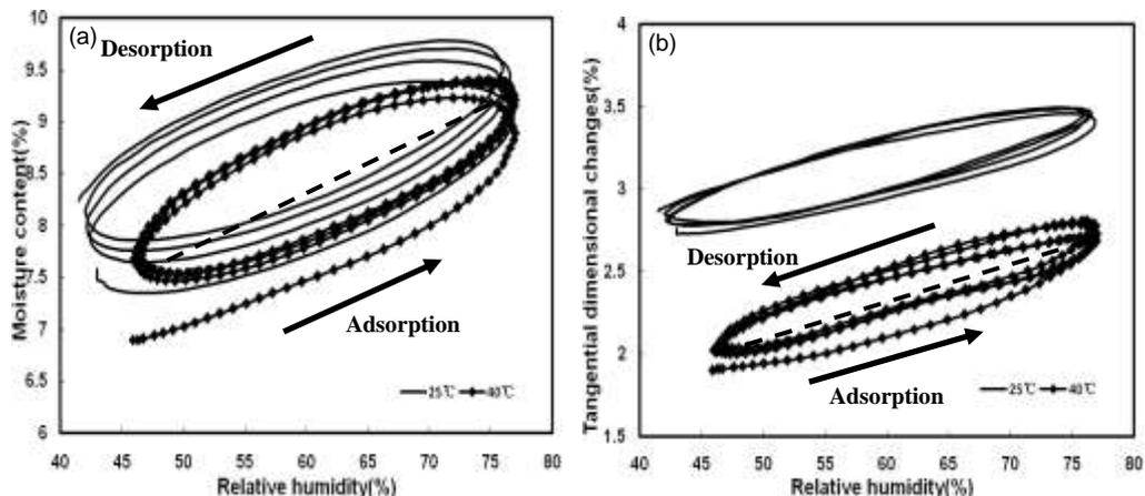
**Fig. 3.** Plots of dynamic sorption isotherms (a) and tangential dimensional changes against relative humidity (b) for 10-mm thick poplar wood cycled for 6 h
