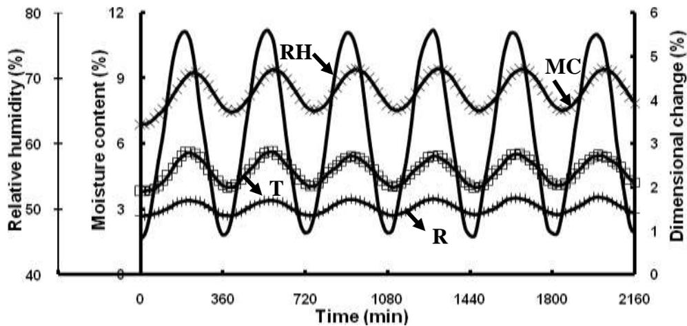
**Fig. 1.** Plots of RH, MC, and R and T dimensional changes against cyclic time for 10-mm thick poplar wood cycled at 6 h at 40 °C
