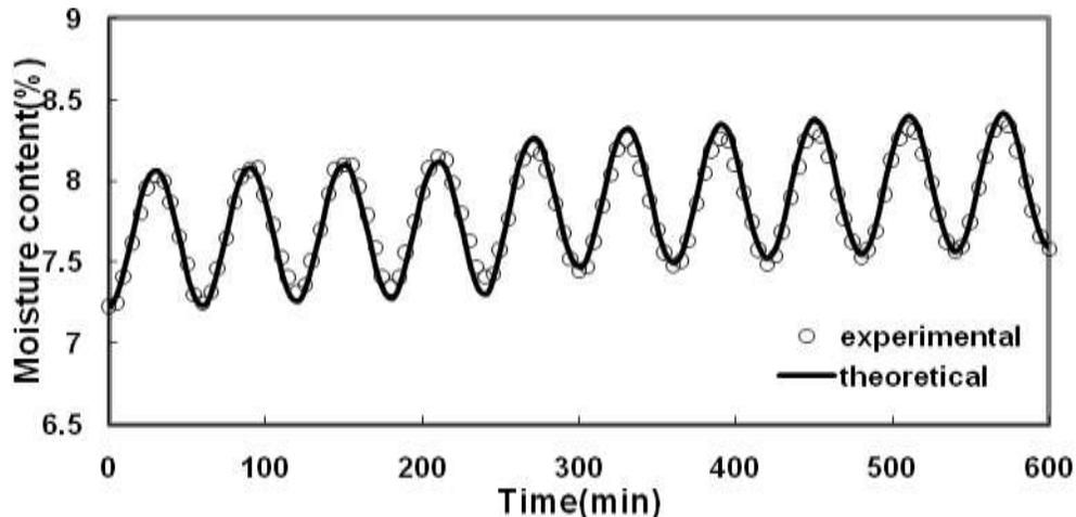
**Fig. 5.** Comparison of theoretical curves with experimental results of dynamic sorption for 10-mm thick poplar wood cycled at 1 h (40 °C)
