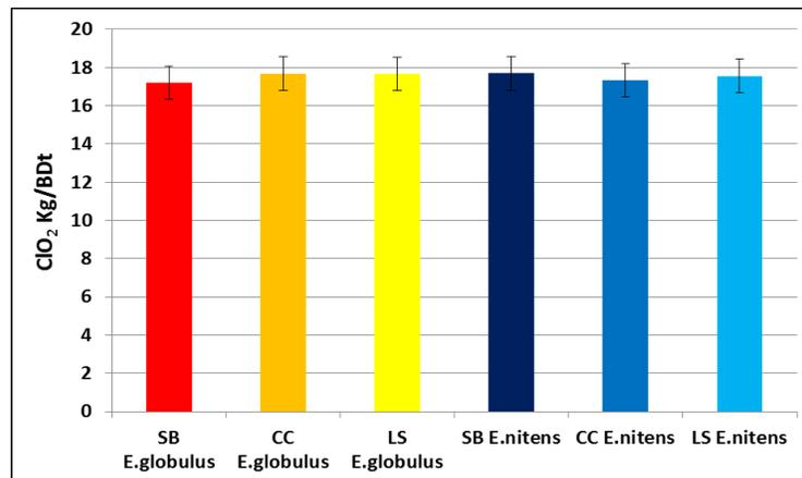
**Fig. 9.** Total  $ClO_2$  consumption to bleach *E. globulus* and *E. nitens* pulps with 95% confidence intervals. The error bars present 95% confidence interval of the mean value.
