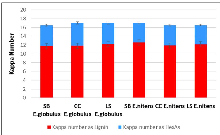
**Fig. 5.** HexA and total lignin of brownstocks representing kappa number  $17 \pm 0.5$  for *E. globulus* and *E. nitens* for the three different cooking methods. The error bars present 95% confidence interval of the value.
