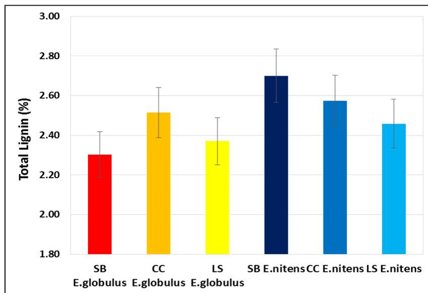
**Fig. 3.** Total lignin in % of brownstocks at kappa  $17 \pm 0.5$ . The error bars present 95% confidence interval of the mean value.
