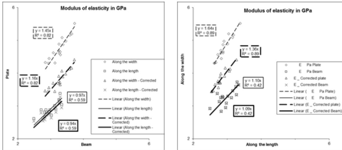
Fig. 5. Comparing the smallest plates (MDF3) with the prismatic beams (MDF4), with and without Brancheriau’s correction coefficient
