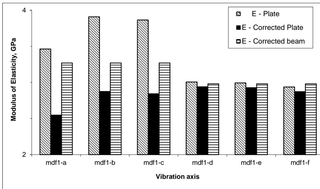
**Fig. 7.** Comparing vibration axes along the width and length. a, b, and c correspond to vibration along the width; d, e and f along the length. Brancheriau's correction coefficient was successfully homogenized the obtained results in whole plate vibration.
