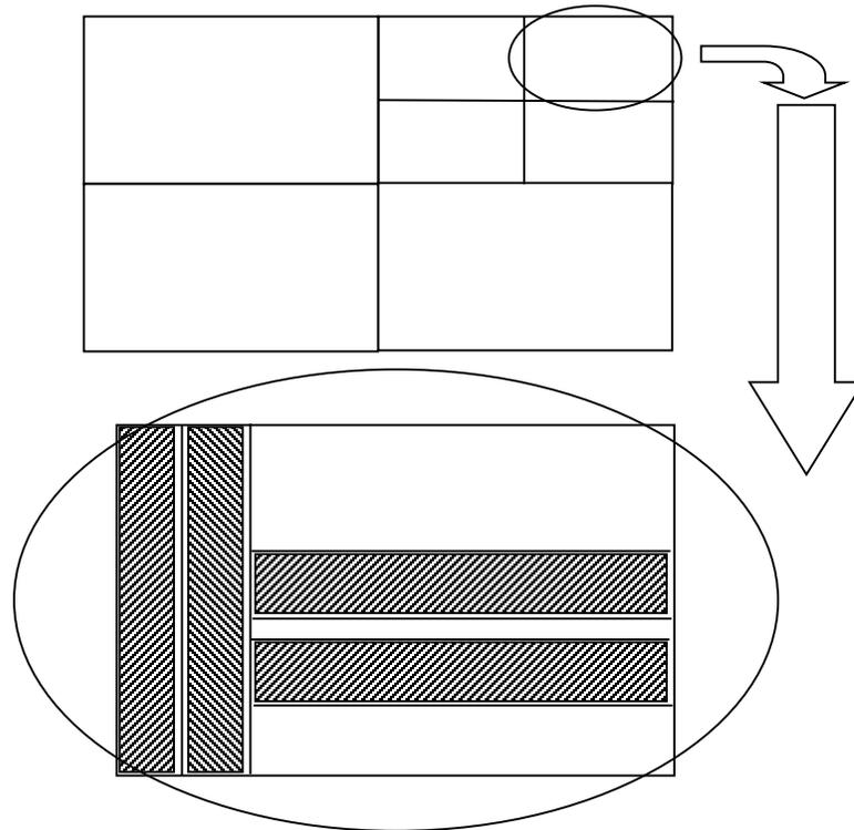
**Fig. 2.** Cutting scenario; the whole plate (MDF1) was divided into 4 (MDF2) then 4 smaller plates (MDF3) and then 4 prismatic beams with lengths oriented individually along the length or width of the whole panel (MDF4)
