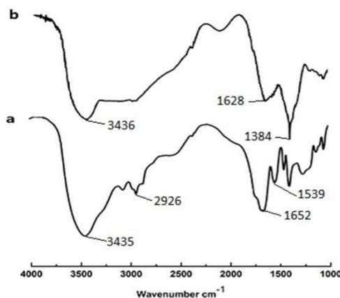
Fig. 2. FTIR spectra of PNVFAA: a: before hydrolysis; b: after hydrolysis
