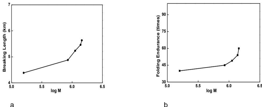
**Fig. 7.** The effect of the molecular weight of P(VAm-co-NaAA) on the (a) tensile strength and (b) folding endurance of handsheets
