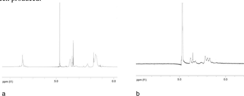
Fig. 3.  $^1\text{H}$  NMR spectra of PNVFAA: a: before hydrolysis; b: after hydrolysis
