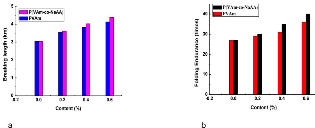
**Fig. 6.** The effect of P(VAm-co-NaAA) content on the (a) tensile strength and (b) folding endurance of handsheets
