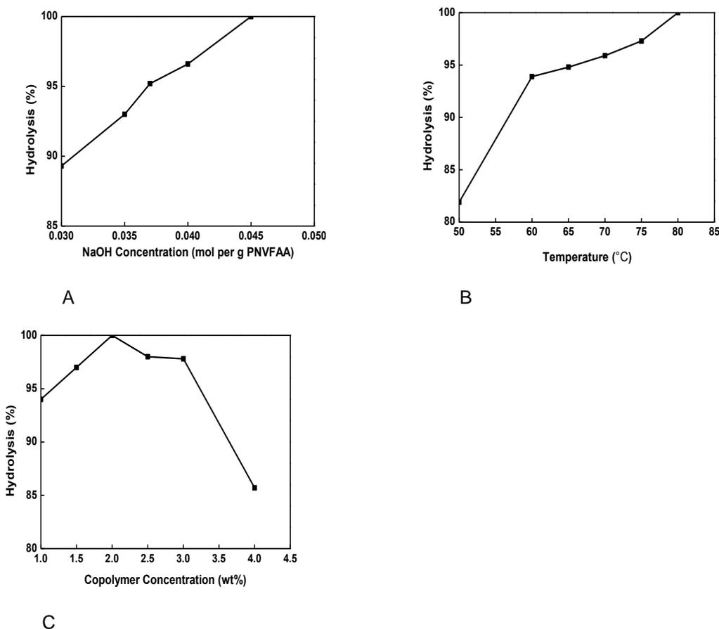
**Fig. 5.** Hydrolysis of PNVFAA varying (A) NaOH concentration, (B) temperature, and (C) copolymer concentration
