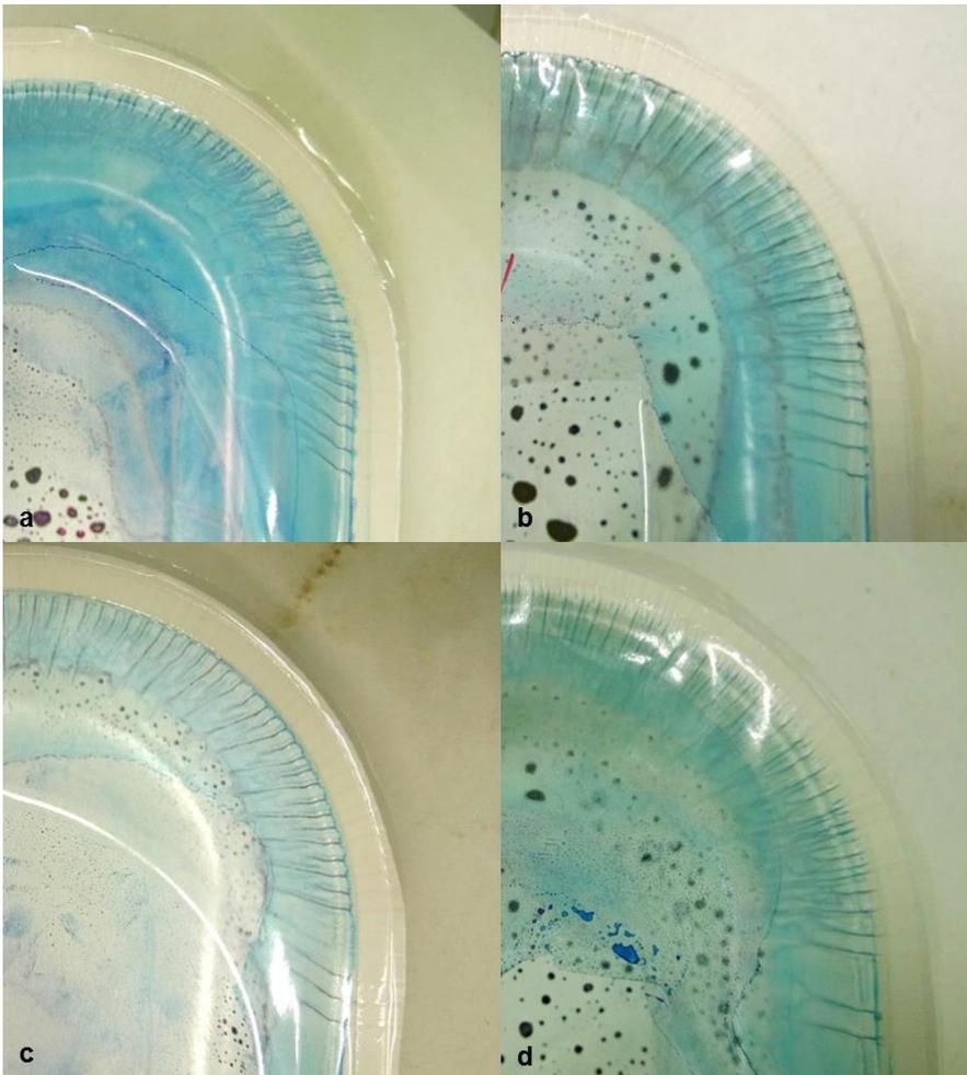
**Fig. 5.** Oval tray corners with different blank holding forces: (a) 1.93 kN, (b) 1.29 kN, (c) 0.94 kN, and (d) 0.52 kN
