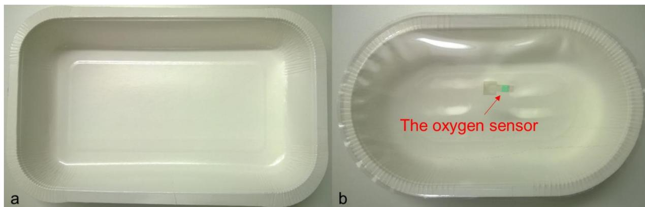
**Fig. 1.** The tray geometries used in the study: (a) rectangular tray and (b) oval tray with the heat sealed lidding film and O<sub>2</sub> sensor
