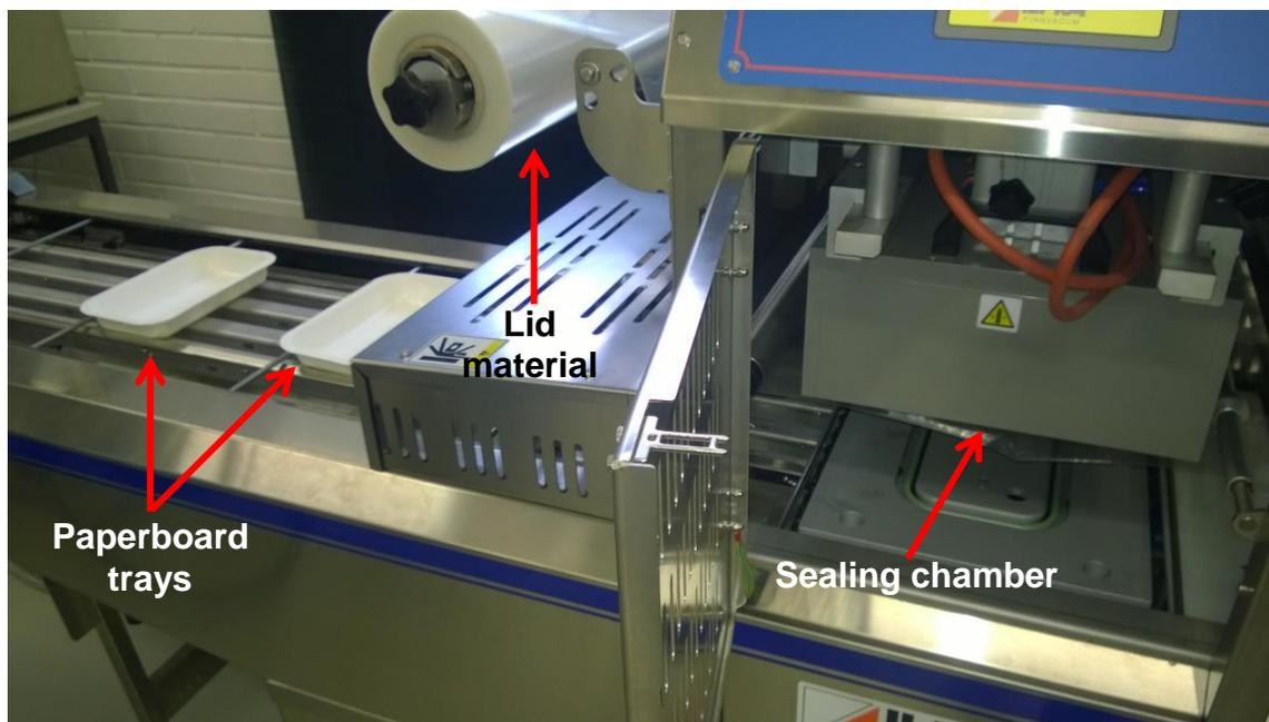
**Fig. 2.** Sealing equipment used in the study
