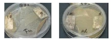
**Fig. 6.** Visual growth of *A. tenuissima* (AI) and *F. culmorum* (Fu) on the surface of wood samples treated with Paraloid B-72 after three months of inoculation at room temperature
