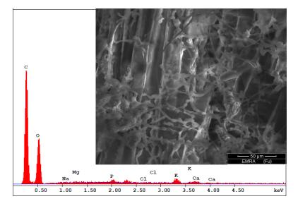
Fig. 2. ESEM and EDX image analysis of the F. culmorum mold on wood
