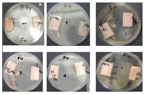
**Fig. 3.** The visual observations for treated *A. saligna* wood with different methanol extracts and Paraloid B-72 with *F. culmorum* (Fu) at different concentrations (5% and 10%). 1- Methanol extract (ME) of *C. sempervirens* wood; 2- ME of *M. pomifera* bark; 3- ME of *M. alba* heartwood; 4-ME of *C. viminalis* bark; 5- ME of *M. grandiflora* leaves
