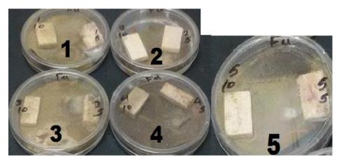
**Fig. 4.** The visual observation of *F. culmorum* growth on the surface of wood samples treated with different extracts and B-72 at the concentrations of 5% and 10% after three months at room temperature. 1- Methanol extract (ME) of *C. sempervirens* wood; 2- ME of *M. pomifera* bark; 3- ME of *M. alba* heartwood; 4- ME of *C. viminalis* bark; 5- ME of *M. grandiflora* leaves
