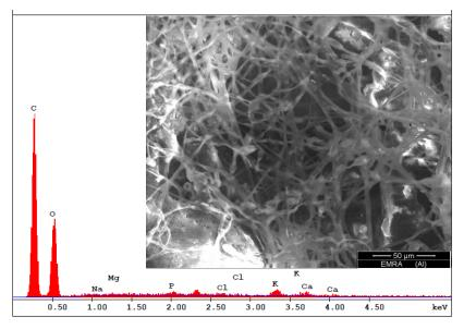
Fig. 1. ESEM and EDX image analysis of the A. tenuissima mold on wood
