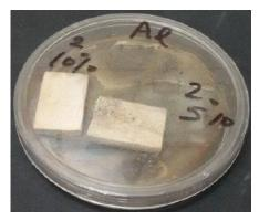
**Fig. 5.** Visual growth of *A. tenuissima* (AI) on the surface of wood samples treated with methanol extract *of M. pomifera* bark after three months at room temperature
