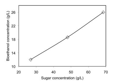
**Fig. 3.** Function describing equation 1 for the sugar concentration against the bioethanol concentration (Design Expert 7.0.0)
