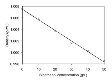
Fig. 1. Calibration curve using coffee mucilage as medium
