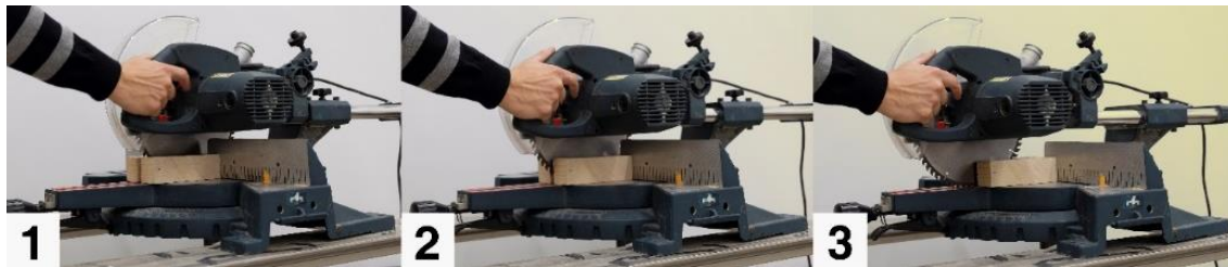
Fig. 6. Sequential saw blade movement through the sample with manual feeding on the sliding mitre saw
