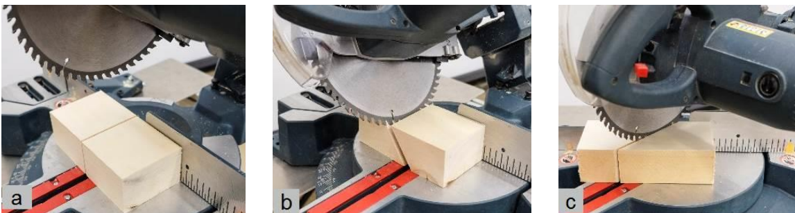
Fig. 8. Cutting orientation of samples: (a) flatwise cross-cutting at \varphi_2 = 90^\circ ; (b) flatwise edge-mitre cross-cutting; and (c) flatwise mitre cross-cutting at \varphi_2 = 45^\circ
