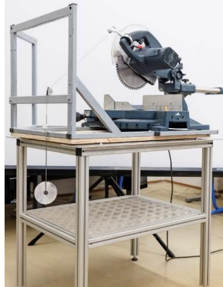
Fig. 5. Experimental stand simulating feed force
