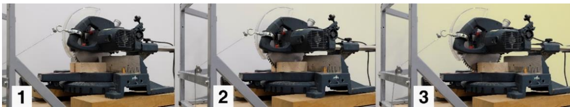
Fig. 7. Sequential saw blade movement through the sample with feeding on the sliding mitre saw by means of the experimental stand
