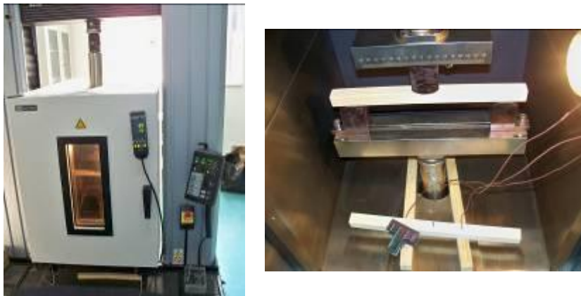
Fig. 1. Test setup for bending strength
