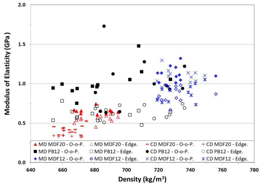
**Fig. 5.** Modulus of elasticity for the square beams cut from large sheet of material along the longitudinal (MD) direction and cross-wise (CD) direction of the panel. The panels include 20 mm thick MDF, 12 mm thick PB, and 12 mm thick MDF. Each beam was oriented with the surfaces of the beam out-of-plane and edgewise with the loading direction.
