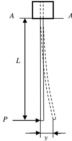
**Fig. 1.** Cantilever beam bending displacement, and resulting load for wood-composite materials
