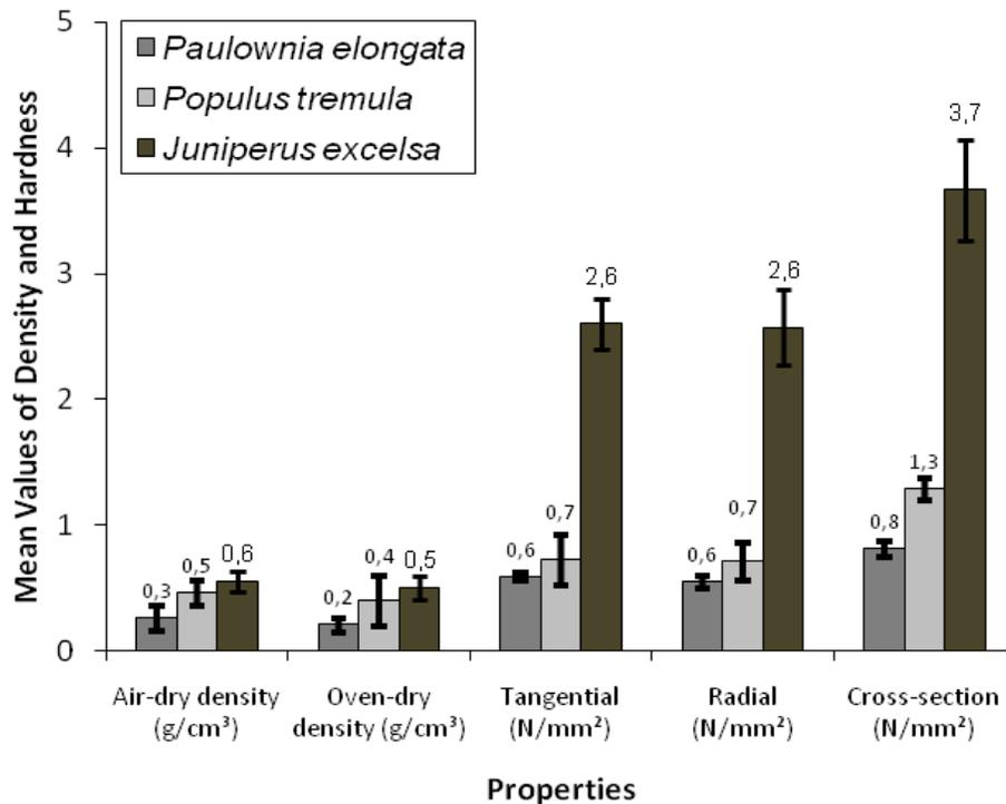
**Fig. 1.** Mean values of density (air-dry and oven-dry) and Brinell hardness (tangential, radial, and cross-sectional)
