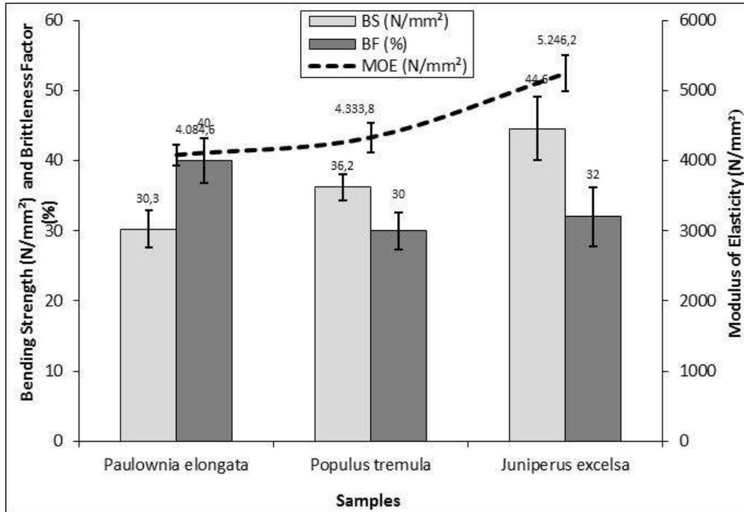
**Fig. 2.** Mean estimates for bending strength (BS), modulus of elasticity (MOE), and brittleness factor (BF)
