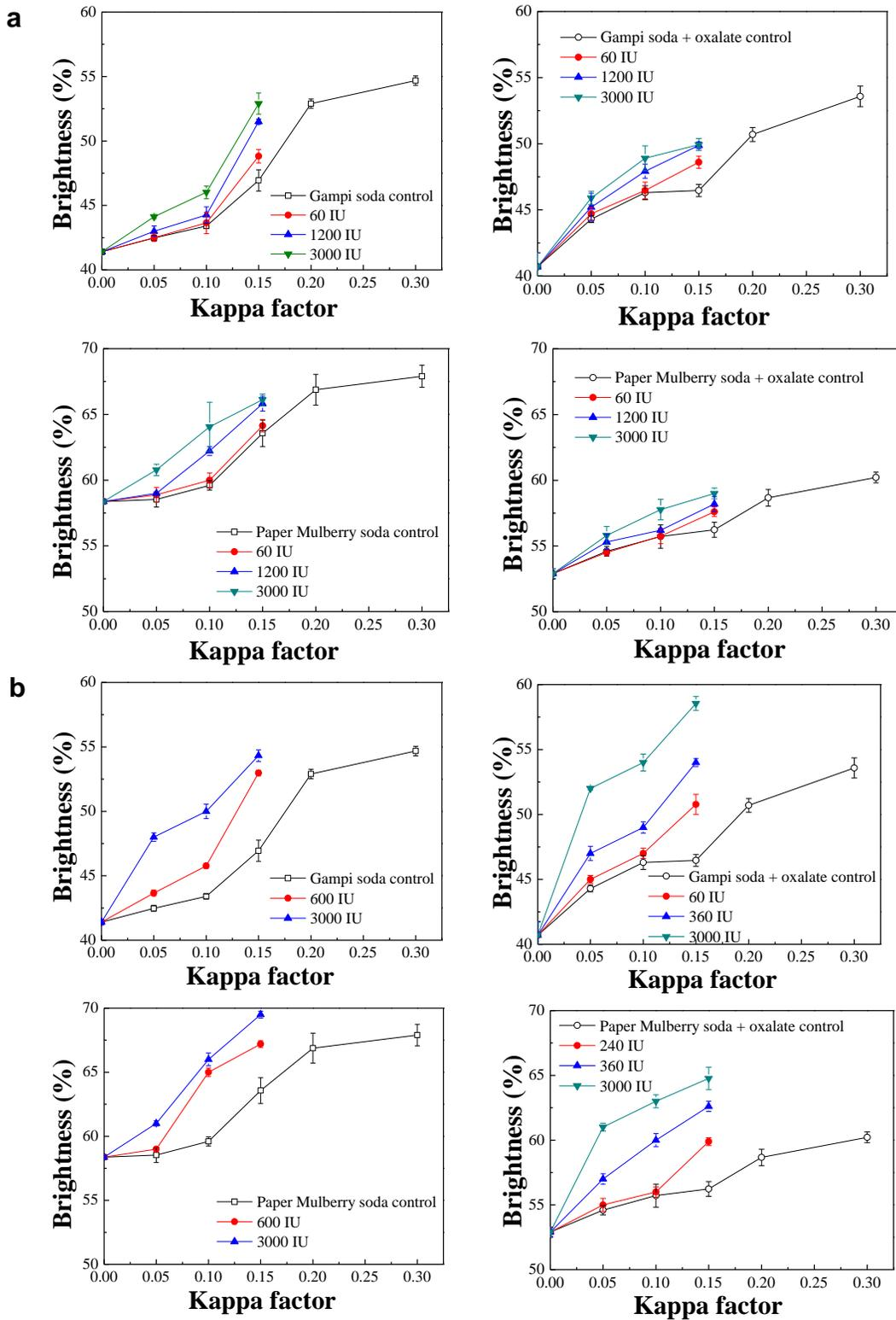
**Fig. 1.** Impact of different dosages of (a) xylanase and (b) pectinase on the brightness of pulp. Data provided as the mean of triplicate  $\pm$  the standard deviation
