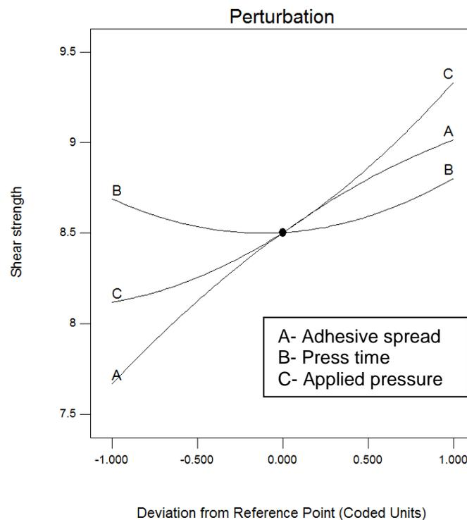
Fig. 2. Perturbation plots showing the effect of each process parameter on the shear strength
