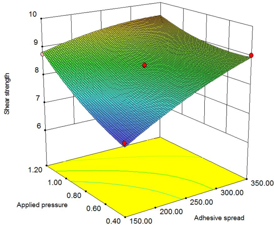
**Fig. 3.** Responses for shear strength as function of major process parameters
