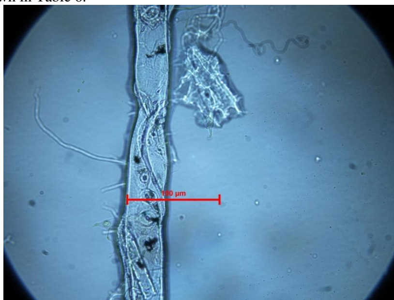
Fig. 4. Microscopic image of a representative newspaper softwood fiber (scale = 100 μm)
