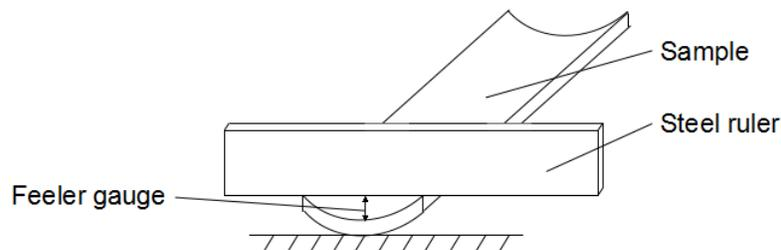
Fig. 5. The picture of warping measurement
