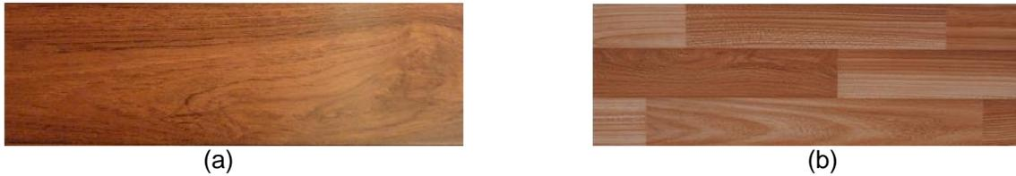
**Fig. 3.** The two shapes of decorative veneers: (a) mono-block and (b) three splice.
