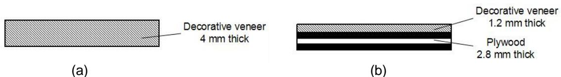
**Fig. 2.** The two structures of the surface layers when the substrate layer was 9 mm thick poplar panel
