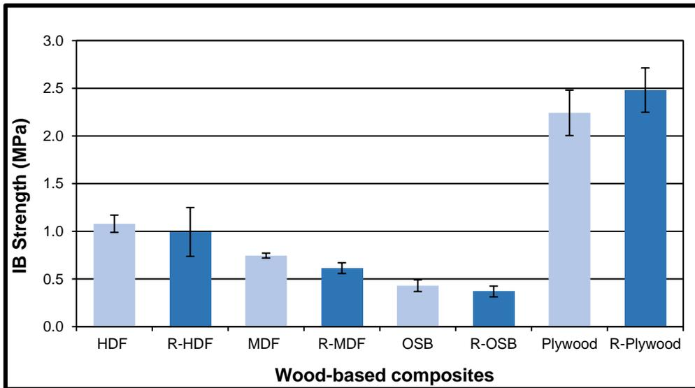
**Fig. 6.** IB strength values of laminated panels and wood-based composites without lamination. IB strength values are the average of 12 replications for each laminated panel and of nine replications for each wood-based composite without lamination.
