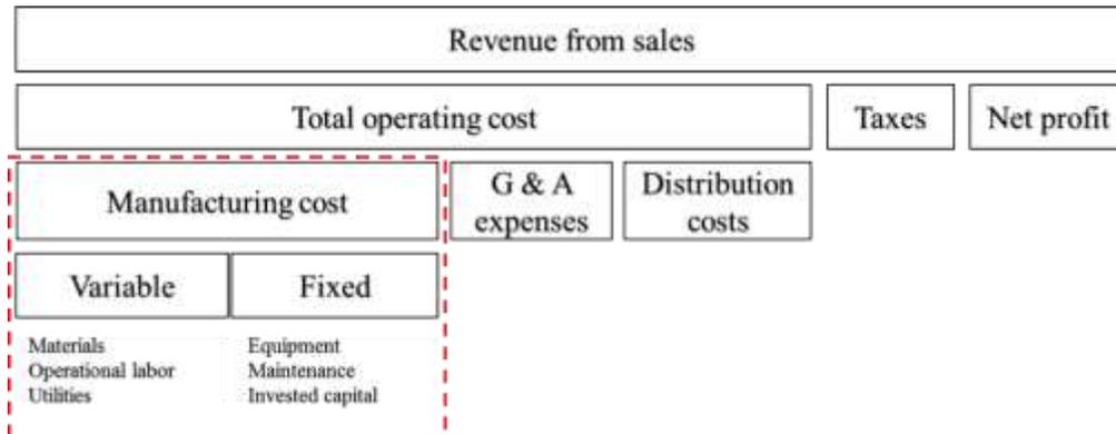
**Fig. 2.** Approach for estimation of manufacturing cost of aluminum-laminated panels
