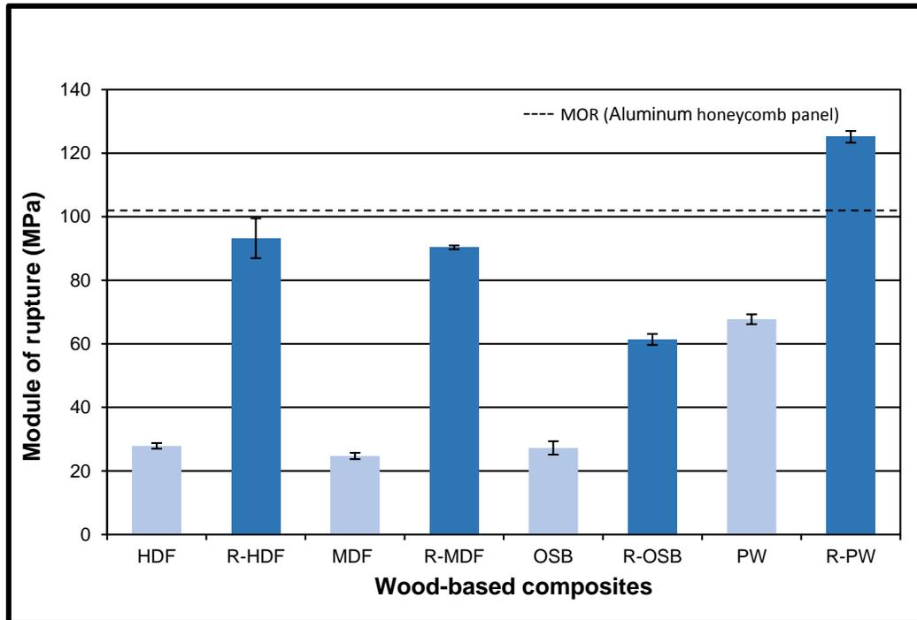
**Fig. 5.** Effects of aluminum alloy sheets on the MOR of wood-based composites. MOR values are an average of 12 replications for each aluminum-laminated panel and of six replications for each wood-based composite without lamination.
