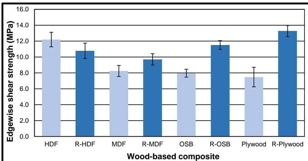
**Fig. 7.** Effect of aluminum alloy sheets on the edgewise shear strength of wood-based composites. Edgewise shear values are an average of eight replications for each laminated panel and wood-based composite without lamination.
