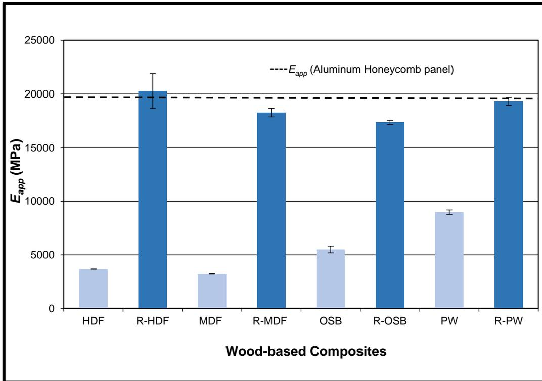
**Fig. 4.** Effects of aluminum alloy sheets on the  $E_{app}$  of wood-based composites.  $E_{app}$  values are the average of 12 replications for each laminated panel and of six replications for each non-laminated wood-based composite.
