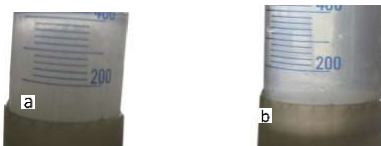
Fig. 3. Drained water containing fines and shortened fibers (a) using the ERD method, along with no fines (b) using the RED method
