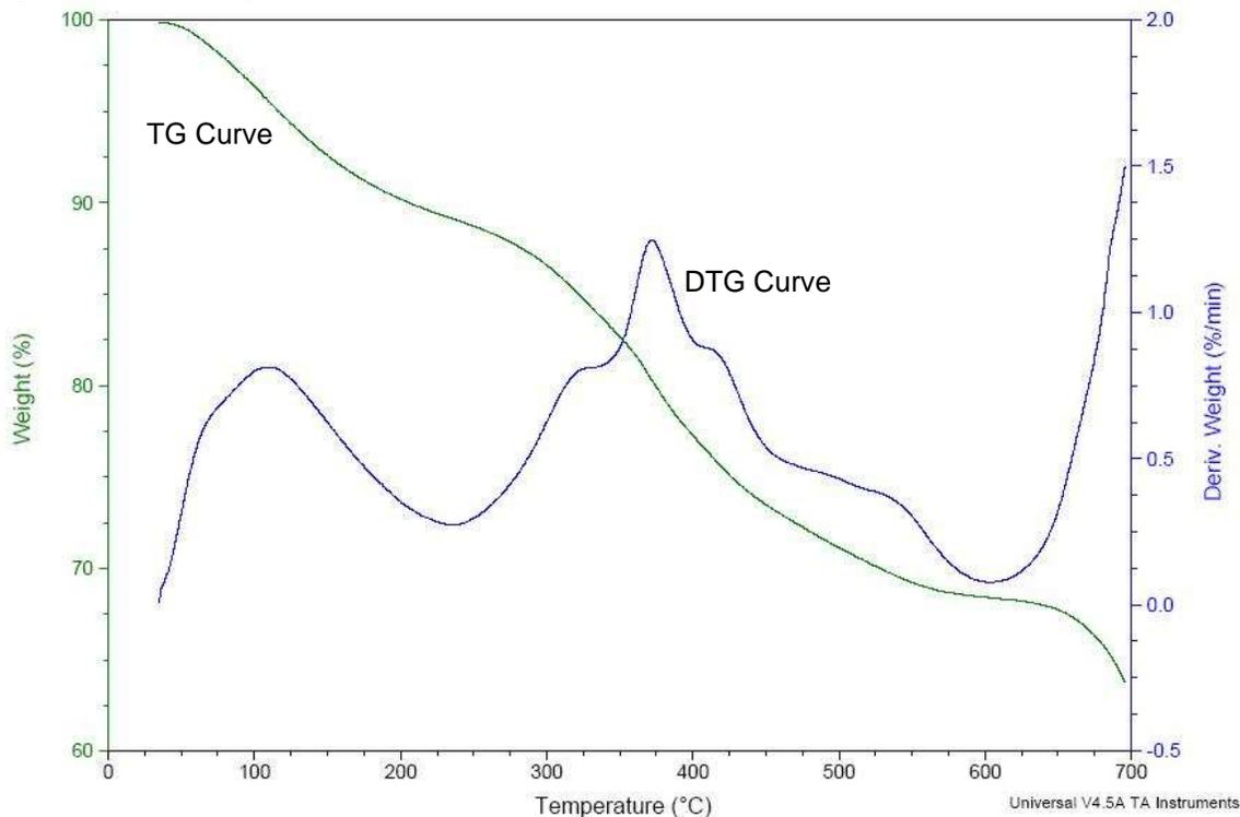
Fig. 2. TGA thermogram of R2 sample
