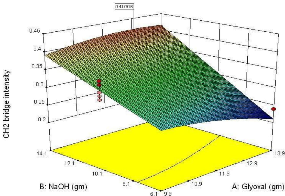
**Fig. 4.** 3D-surface plot of intensity of relative absorbance for CH<sub>2</sub> bridges in glyoxalated lignin as a function of weights of glyoxal and NaOH
