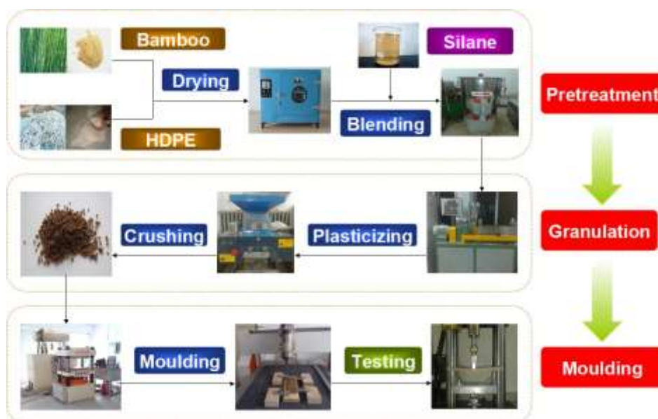
Fig. 1. Technological roadmap of proposed silane KH550 surface modified moso bamboo flour/HDPE composite engineering material
